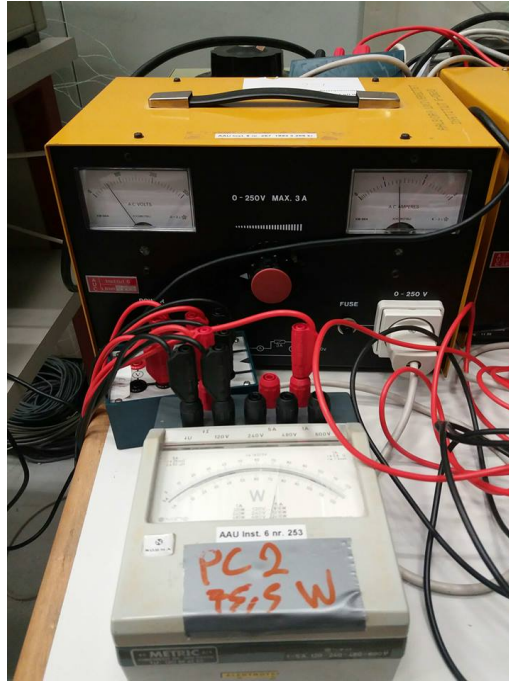
Figure B.2. RKT-2 voltage regulator combined with a HEWa-21 watt-meter
