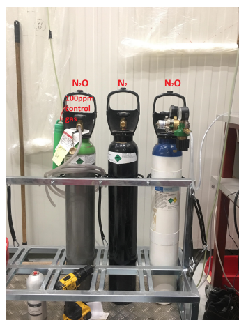
Figure 5.6. Gases used for the experiment and equipment control test
