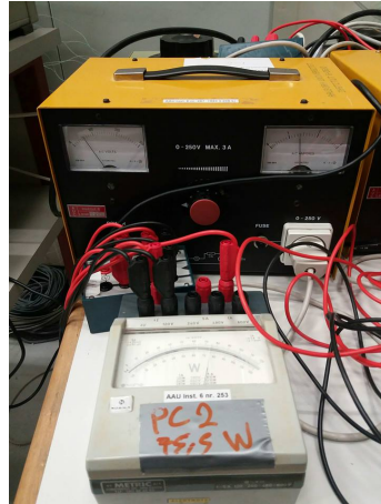
Figure 5.5. RKT-2 voltage regulator combined with a HEWa-21 watt-meter
