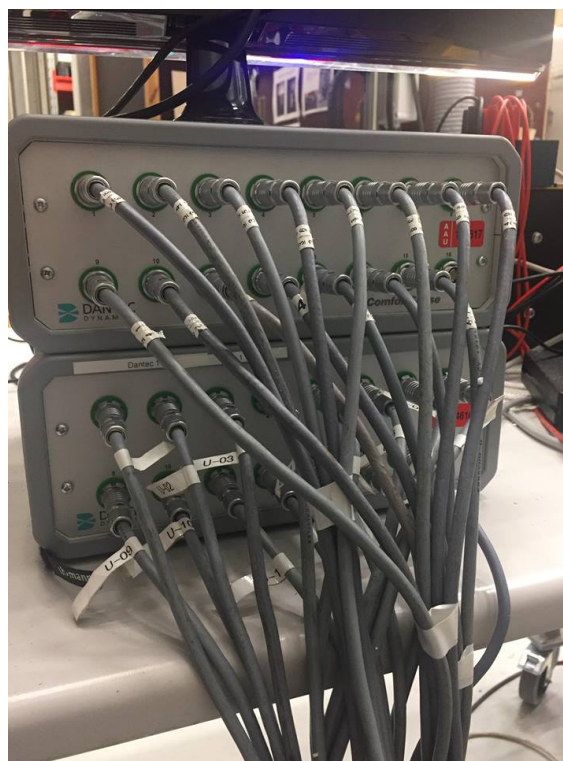
Figure C.9. Comfortsense connected to the anemometer cables.
