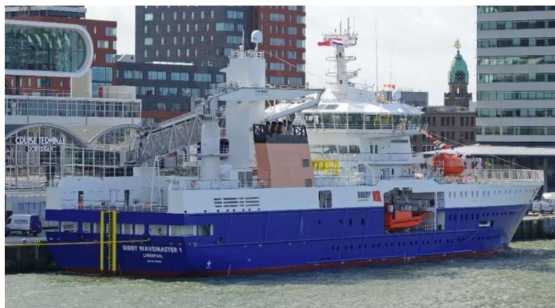
Figure 2.5: SOV BIBBY WAVEMASTER 1 equipped with a W2W system. Source: [16]
