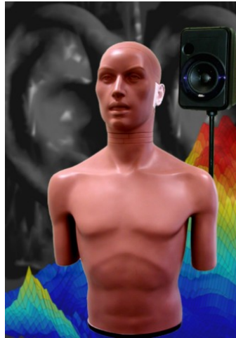
Figure 9: Example of mannequin for binaural recording
