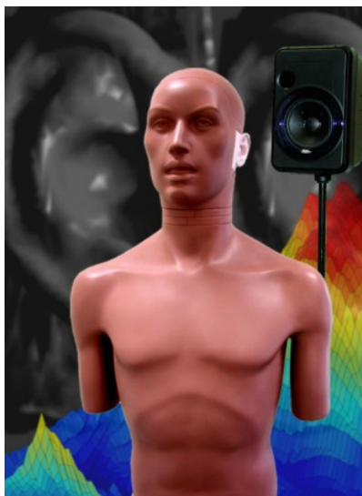
Figure 29: Example of mannequin for binaural recording
