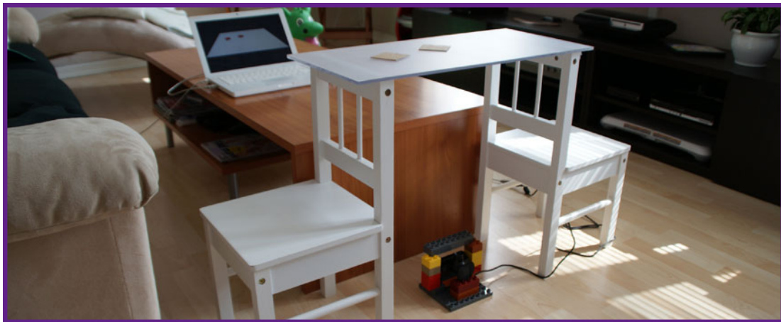
Figure 29 - Early prototype setup: Cardboard objects, surface on chairs & camera mounted on LEGO.
