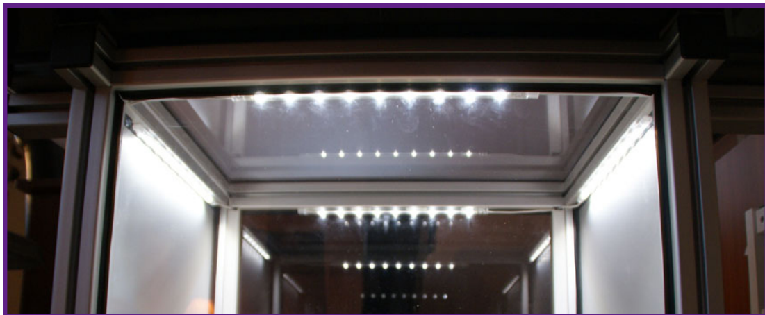
Figure 31 - The underside of the tabletop surface, illustrating the positioning of the LED arrays.
