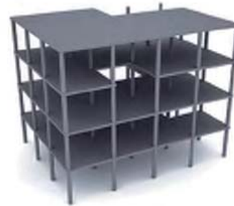
Ill. 17: The column/slab system. It gives more freedom for the spatial organising.
