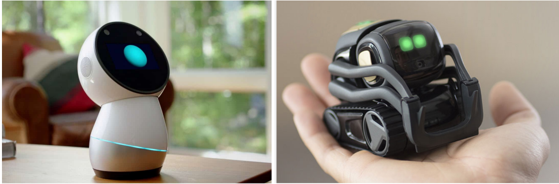
Figure 2.3. Examples of consumer social robots. To the left, Jibo. It has facial recognition and natural language processing. To the right is the Vector robot which is mobile and designed to be a little desktop helper. Jibo picture from https://aiscores.com/jibo/ , Vector picture from https://www.anki.com/en-us/vector/vector-aware.html - Accessed 2019-05-02.
