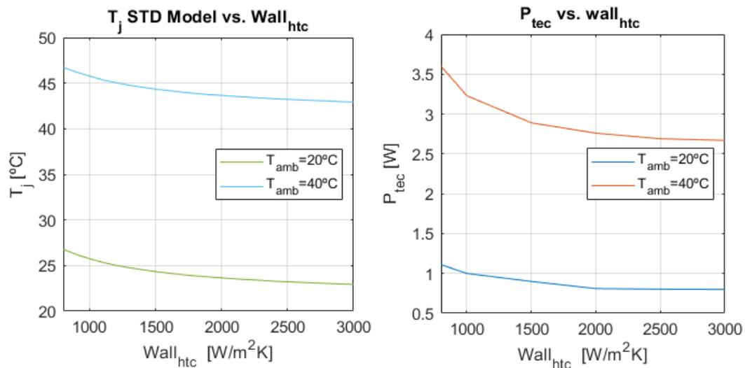
**Figure 5.10:**  $T_j$  at STD model (left).  $P_{tec}$  consumed by the TEC to keep a  $T_j$  of 25°C (right). Heat sink surface:  $34 \cdot 30 \text{ mm}^2$
