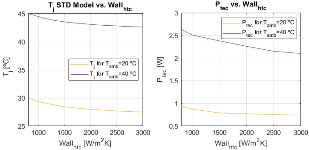
**Figure 5.11:**  $T_j$  at STD model (left).  $P_{tec}$  consumed by the TEC to keep a  $T_j$  of  $25^\circ\text{C}$  (right). Heat sink surface:  $40 \cdot 40\text{mm}^2$
