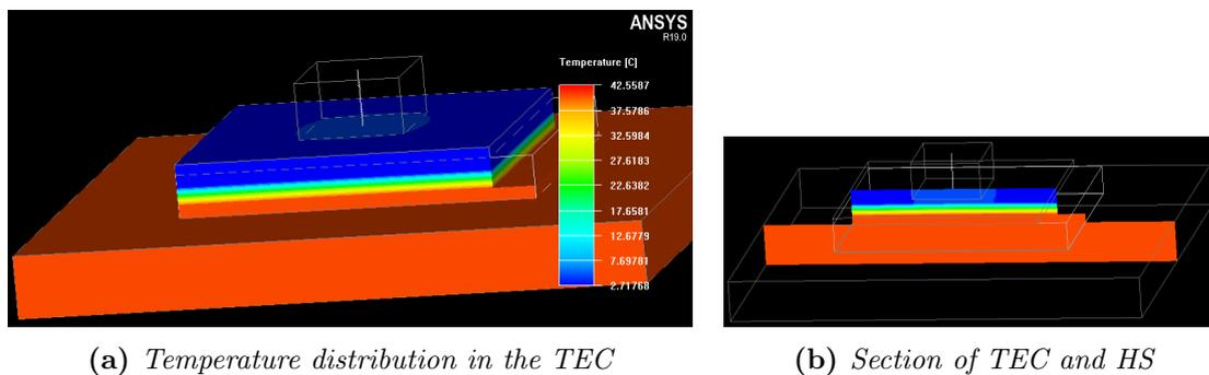
**Figure 5.7:** Results of temperature distribution on the TEC system in Icepak
