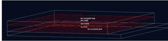
Figure 4.4: TEC model in Icepak represented by two ceramic plates at top and bottom, two sources to simulate the conduction plates and a solid block representing the thermoelectric material of the TEC
