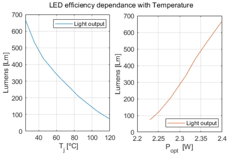
**Figure 3.8:** *Luminous flux vs.  $T_j$  (Left). Luminous flux vs.  $P_{elec}$  (right). Both graphs represent the relation between the Lumens,  $T_j$  and  $P_{opt}$  for  $I_f = 3.15A$  and  $\eta_e = 0.34$ .*
