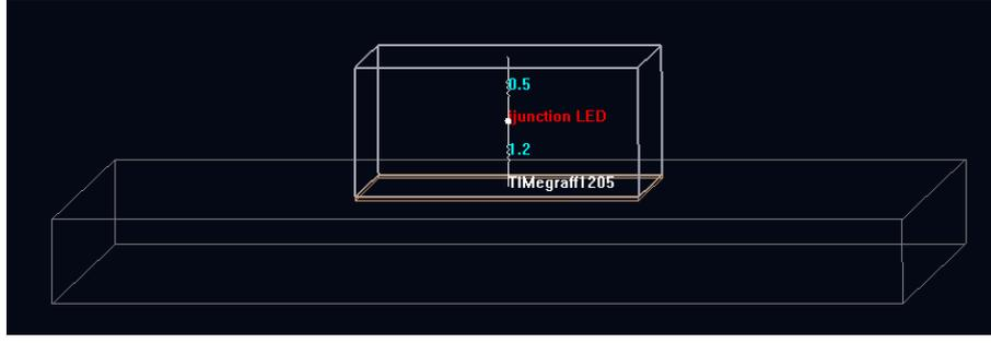
**Figure 3.5:** Complete STD LED model at Icepak. Network block (defining the  $R_{jc} = 0.5$ ,  $R_{jb} = 1.2$ ,  $P_h = 4.215$ ), conducting plate as TIM, HS of  $40 \cdot 40 \text{mm}^2$  and the wall ( $Wall_{htc}$ ), not visible here, to define the heat transfer coefficient on the bottom surface of the HS respect to  $T_{amb}$
