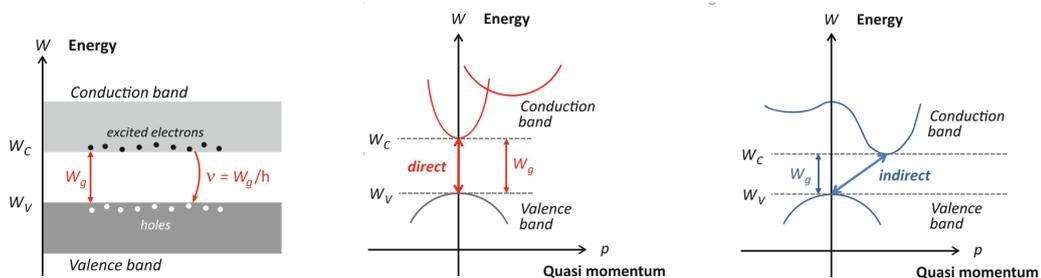
Figure 3.1: Band structure [Editors and Thermal]
