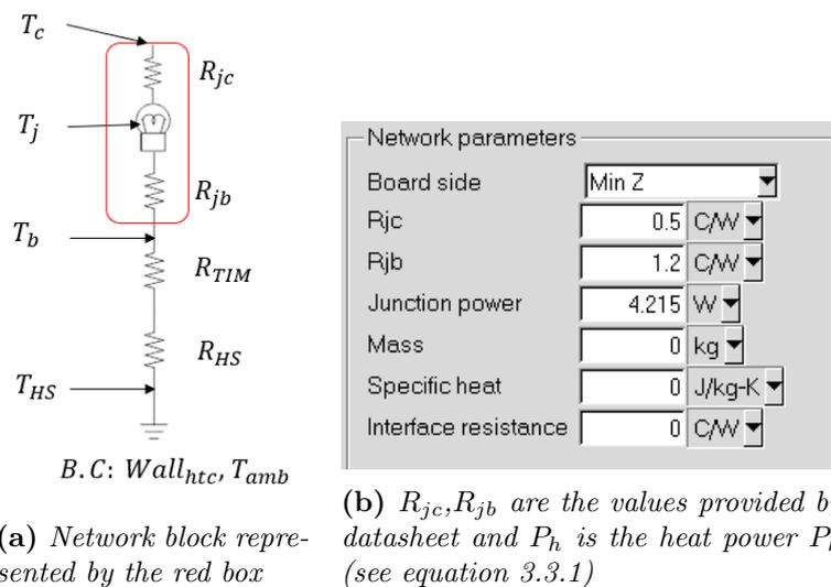
**Figure 3.4:** Compact two resistor model LED:  $T_j$  is the junction temperature,  $T_c$  is the case temperature,  $T_b$  represents the temperature at the bottom of the MC PCB and  $T_{HS}$  defines the temperature at the base of the HS. Boundary conditions (B.C):  $Wall_{htc}$  and  $T_{amb}$
