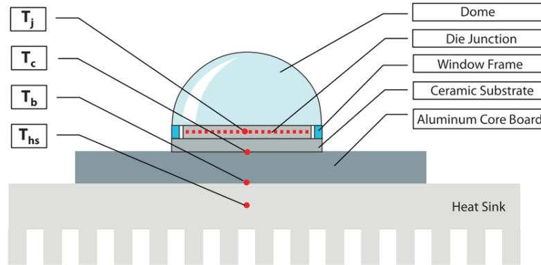
**Figure 3.3:** Typical thermal resistances [Shipping et al., 2015]
