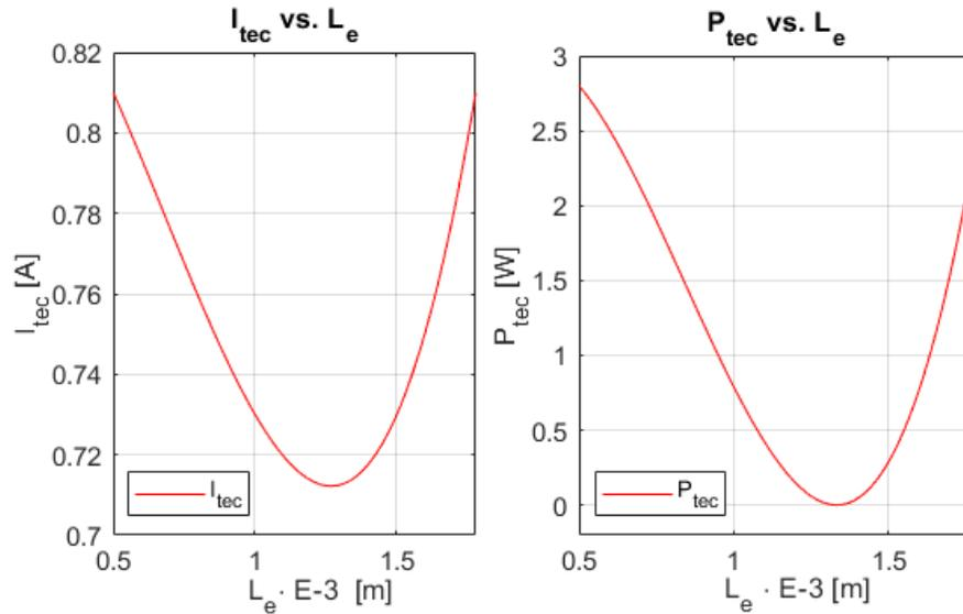
**Figure 5.9:** Current and power against different thermoelement longitudes for  $Wall_{htc} = 1500 \text{ W/Km}^2$  for  $T_{amb} = 40^\circ \text{ C}$
