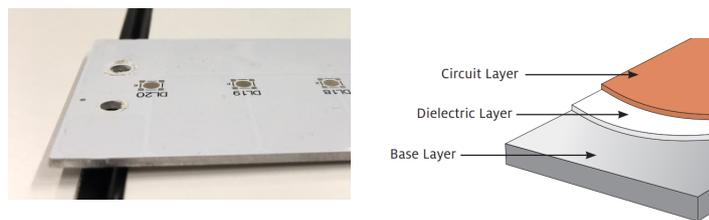
**Figure 3.2:** *MC PCB [Guide]*
