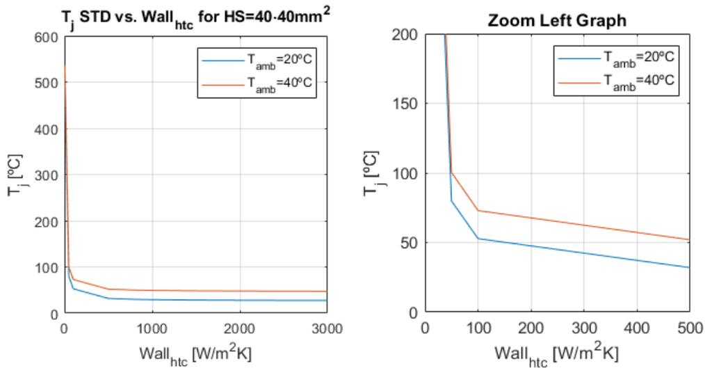
**Figure 5.2:** Temperature distribution for different  $Wall_{HTC}$  and different  $T_{amb}$  and a HS surface of  $34 \cdot 30 \text{ mm}^2$
