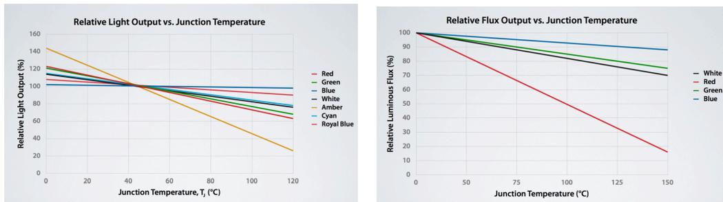
**Figure 1.2:** Performance dependency of temperature of different LED colours [Gala, 2017]
