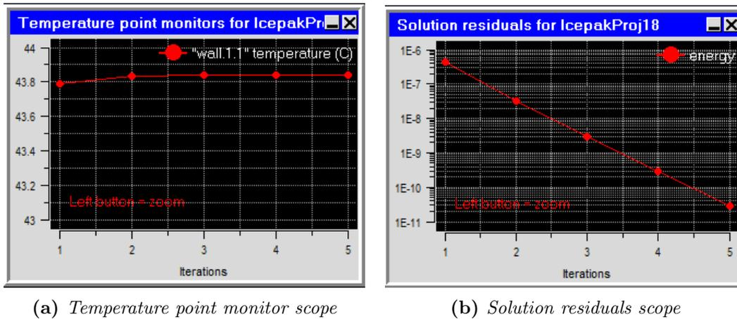
**Figure 3.6:** Monitoring solution process in Icepak
