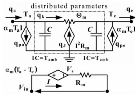
**Figure 1.3:** *Distributed TEC system in Spice[Lineykin and Ben-Yaakov, 2005]*
