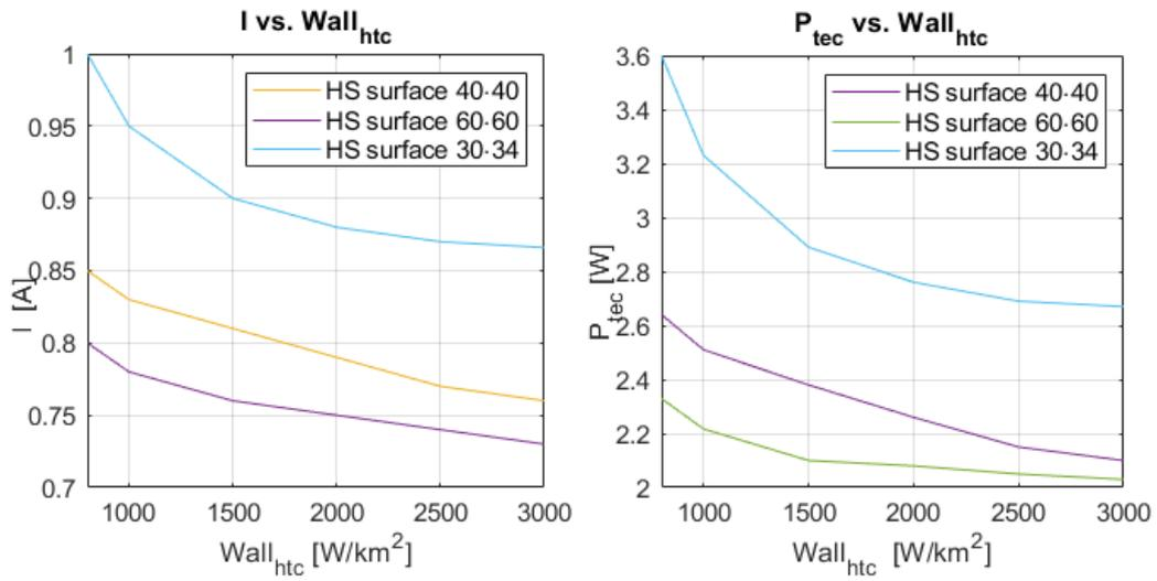
**Figure 5.8:** Current and power against different  $Wall_{htc}$  for  $T_{amb} = 40^{\circ}C$
