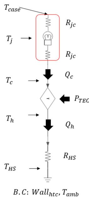
**Figure 4.5:** Network thermal TEC model representing the thermal resistances, temperatures and power fluxes occurring in the TEC system
