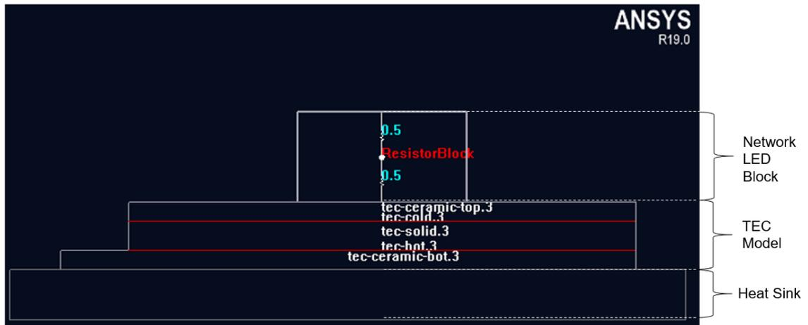
(a) 2D model of the TEC system for  $HS = 40 \cdot 40\text{mm}^2$
