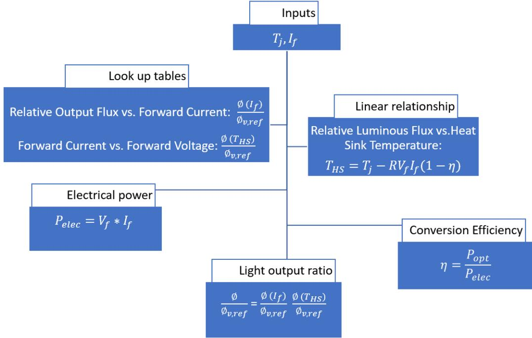
**Figure 3.7:** Schema describing the process to obtain Light output
