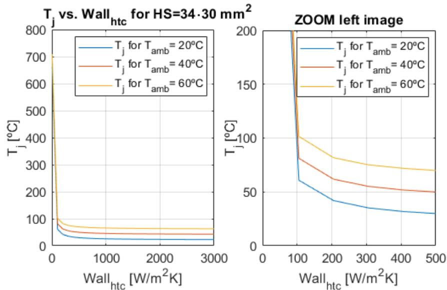
**Figure 5.1:** Temperature distribution for different  $Wall_{HTC}$  and different  $T_{amb}$  for a HS surface of  $40 \cdot 40 \text{mm}^2$
