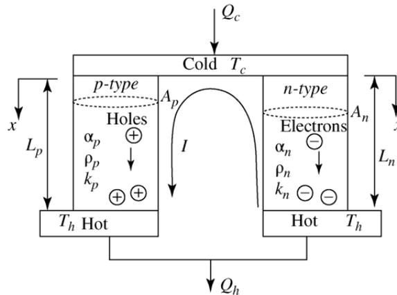
**Figure A.1:** Thermoelectric couple with two dissimilar materials [Peltier et al., 1960].
