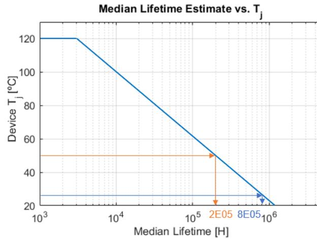
**Figure 3.9:** Median Lifetime Estimate. Lifetime defined as time to 70% of initial intensity [Shipping et al., 2015]
