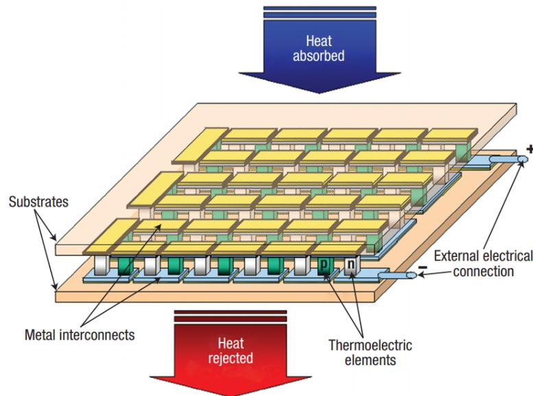
**Figure 4.2:** *TEC module Snyder et al. [2003].*
