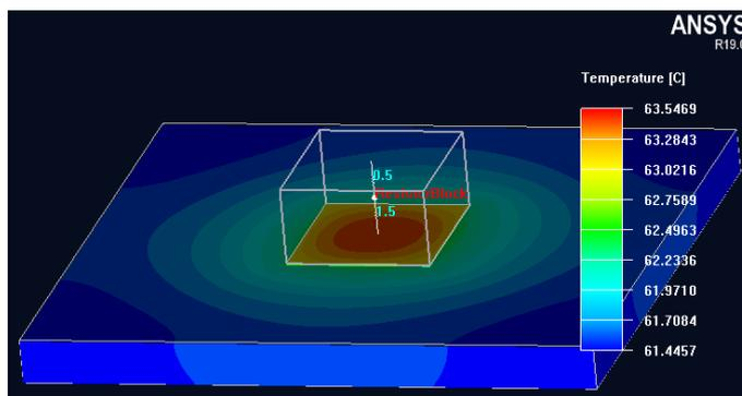
**Figure 5.3:** Distribution temperature for LED model
