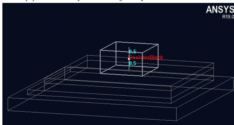
(b) 3D model of the TEC system. The values seen on the figure represents the given  $R_{jc} = 0.5 \text{ K/W}$  available at datasheet.
