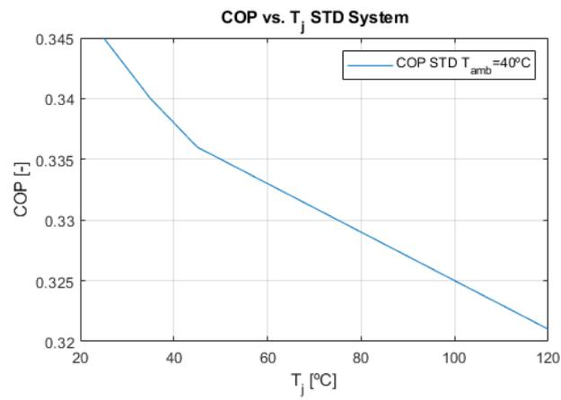
**Figure 5.5:** COP of the Standard LED system as function of  $T_j$
