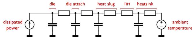
**Figure 1.4:** *Cauer LED Thermal Model [Version and Technology, 2012]*
