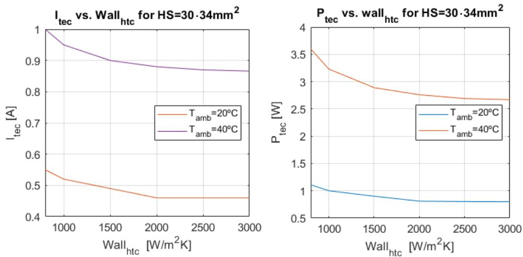
**Figure 5.6:** Current and power against different  $Wall_{htc}$  with a HS surface of 30·34mm<sup>2</sup>
