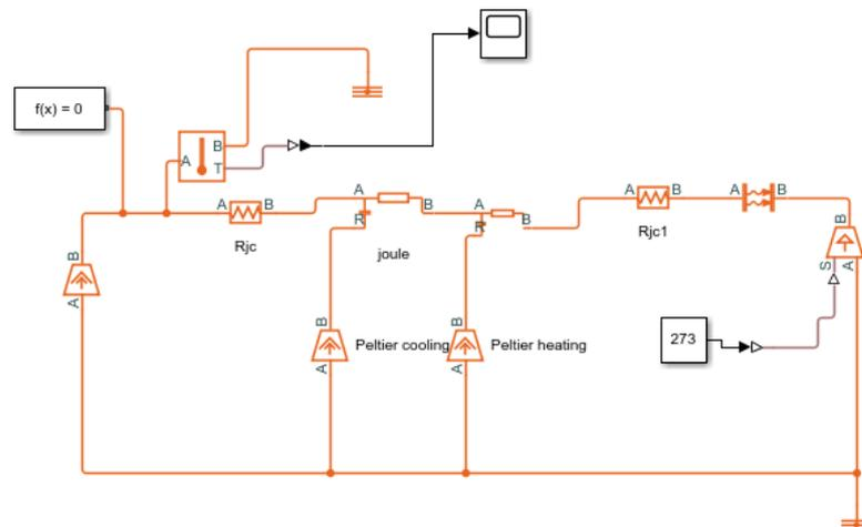
**Figure 7.1:** *Distributed TEC model with Simscape objects*
