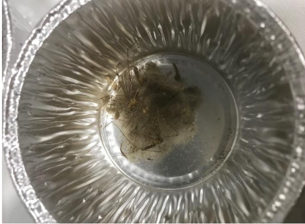
Figure 22. A filter dirt sample with organic material
