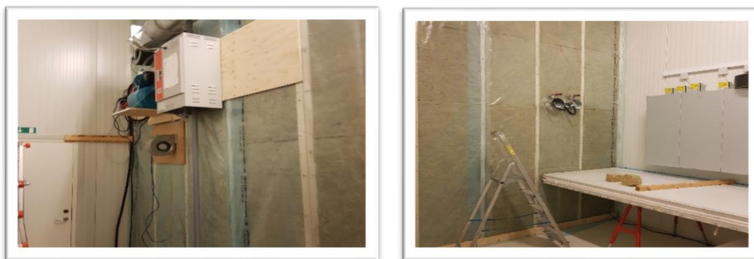
Figure 3. On the left, the test room (climatic chamber, to test filters at different levels of RH. On the right, the cold room for dehumidification.
