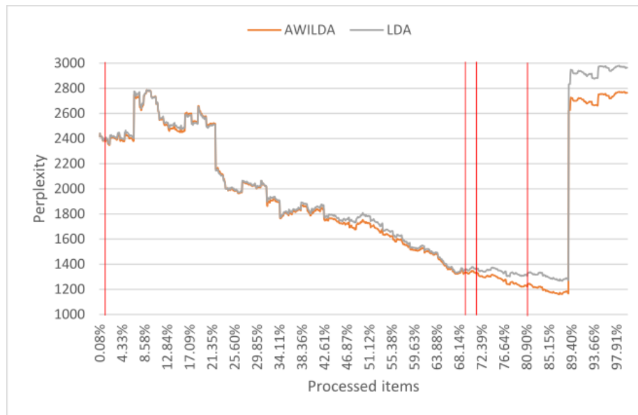
Figure 7.1: Comparison of the performance of AWILDA and online LDA on the O11Intern dataset, measured as the average perplexity of a sliding window. Each red line indicates a drift detected by AWILDA.
