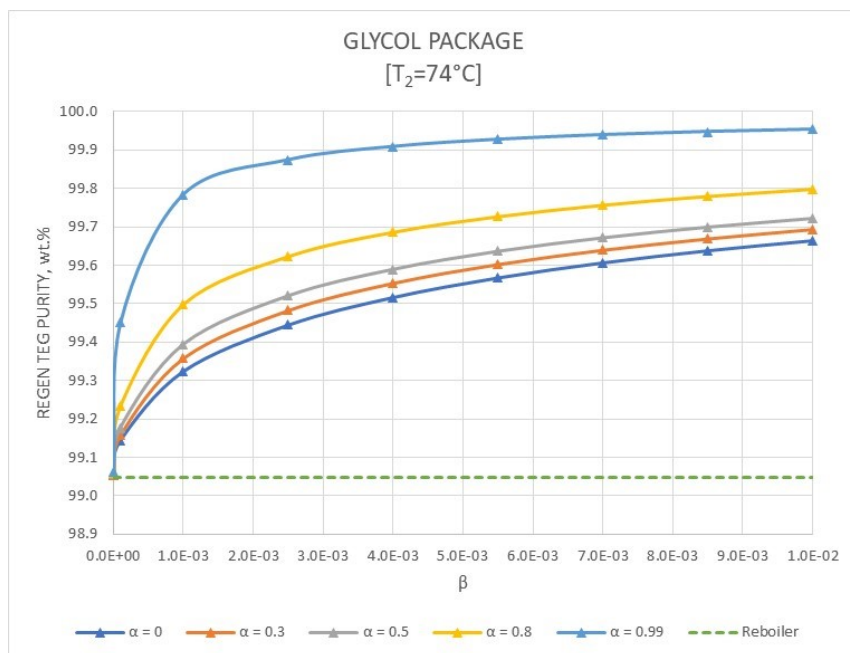
Figure 6.13: Purity of TEG (wt.%) as function of \beta , for different values of \alpha and T_2 = 74^\circ\text{C} obtained with HYSYS ®
