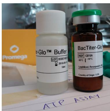
Figure 6: shows two reagents of BacTiter-Glo™, the buffer and the enzymatic cocktail.
