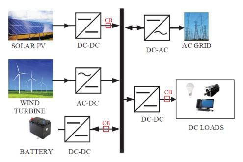
Figure 1.6: Signal bus microgrid with circuit breakers (CB) installed in each of its branches
