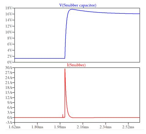
Figure 5.8: Response simulation of the CB (snubber branch)
