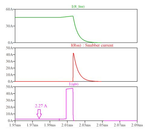
**Figure 4.6:** Green = line current, red = Snubber current, Magenta = IGBT current. Static consumption of 2.27 A
