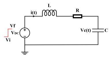
Figure 3.17: An RLC series circuit schematic
