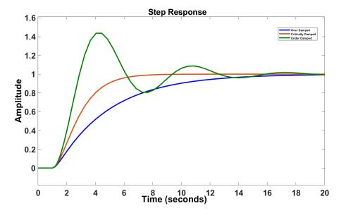
Figure 3.18: Over-Damped, Critically-Damped and Under-Damped response of series RLC circuit
