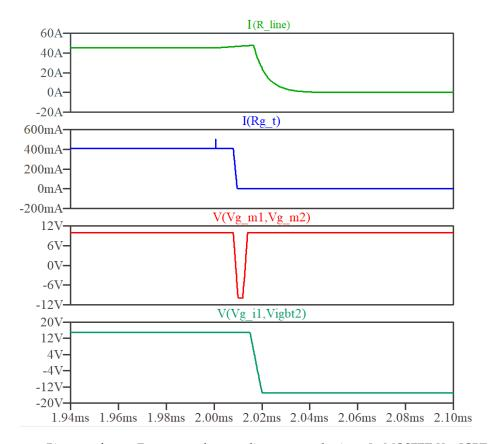
**Figure 4.5:** Bias waveforms. From top to bottom: line current, thyristor  $I_g$ , MOSFET  $V_{gs}$ , IGBT  $V_{ge}$
