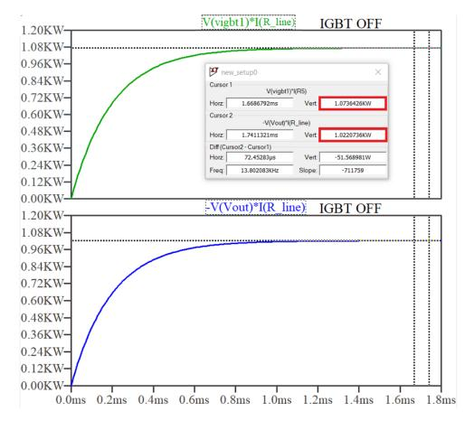
Figure 4.8: Steady-state power loss if the IGBTs remain open until the fault occurs
