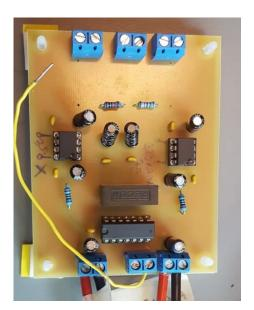
**Figure 5.6:** IGBT driver board. The green and yellow cables conduct the control signal from Arduino to the board.
