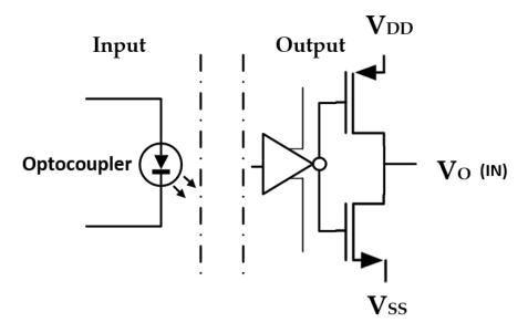
**Figure 3.8:** Isolated gate driver providing electric isolation between input and output.  $V_{DD}$ : positive power supply,  $V_{SS}$ : negative power supply
