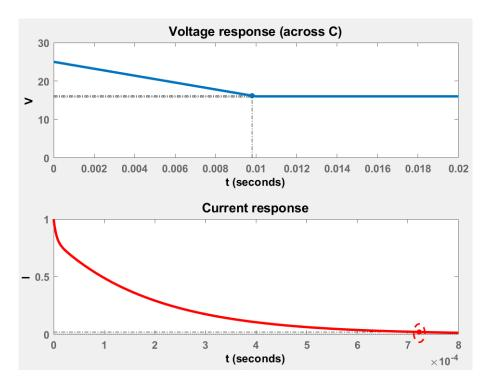
Figure 5.7: Impulse response of the RLC circuit
