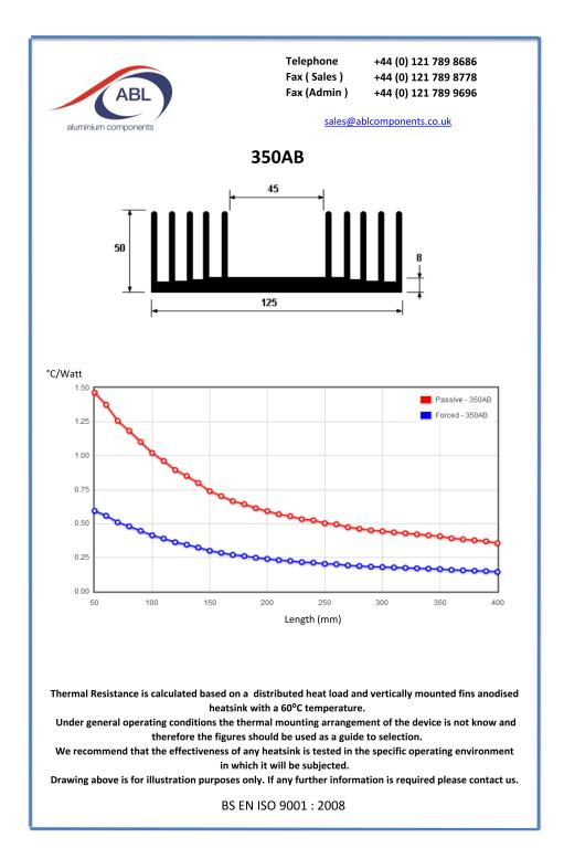
Figure A.4: Attached heatsink to the anti-parallel thyristor module
