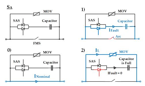
**Figure 1.7:** 0) Normal condition: FMS is closed; 1) Fault condition: FMS in red is open; 2) Capacitor is charged so the thyristor begins to block the voltage. MOV: Metal Oxide Varistor, SAS: Semiconductor Accessary Switch, FMS: Fast Mechanical Switch
