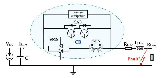
**Figure 3.3:** Selected circuit breaker protecting a microgrid circuit based on a DC source, a line inductance and a resistive load
