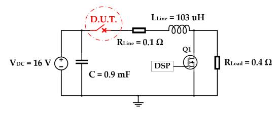
**Figure 6.1:** Common setup. In the red spot will be connected the corresponding circuit breaker under testing
