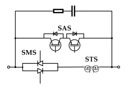
Figure 6.3: Power circuit of the Modern Breaker
