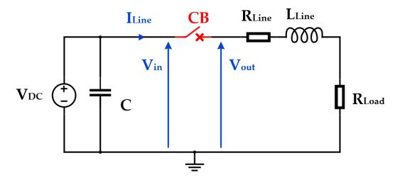
Figure 3.4: Location of the measurements
