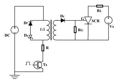
Figure 3.12: Pulse transformer based thyristor gate driver circuit
