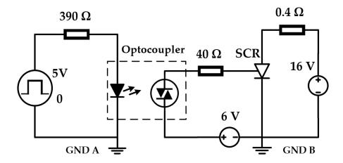
Figure 5.3: SCR gate driver test circuit
