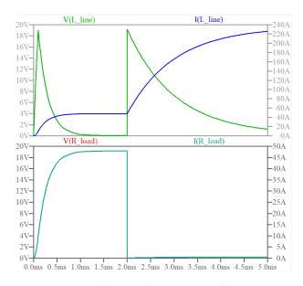
**Figure 4.3:** Fault beginning at 2ms. Voltage and current waveforms across: up) the line inductor, down) the resistive load
