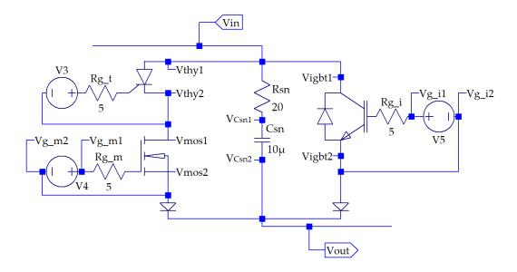
Figure 4.4: Functional model of the circuit breaker
