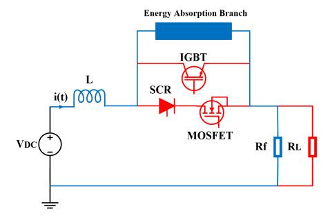
**Figure 3.13:** Last state of the CB. Blue: new current path, Red: no current-flow. Unidirectional case is shown to more easily show the concept
