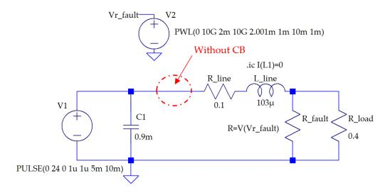
**Figure 4.2:** Circuit modeling a pole-to-ground fault between two terminals in a low voltage microgrid. From left to right: generator, line and consumer ( $R_{load}$ ). The red oval indicates the circuit breaker is not included in the circuit.
