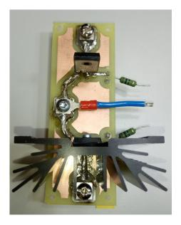
Figure 5.2: Common-source power MOSFET circuit
