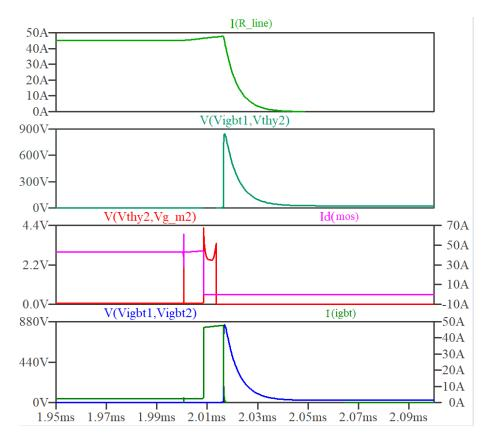
Figure 4.9: Voltages and currents in the circuit breaker
