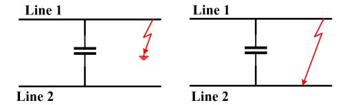
Figure 3.2: (a) Line-ground fault in DC bus, (b): Line-line fault condition in DC bus
