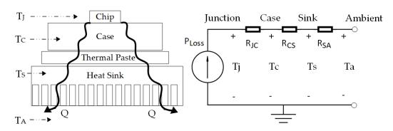
Figure 3.6: Typical power module (left). Steady state thermal model (right).
