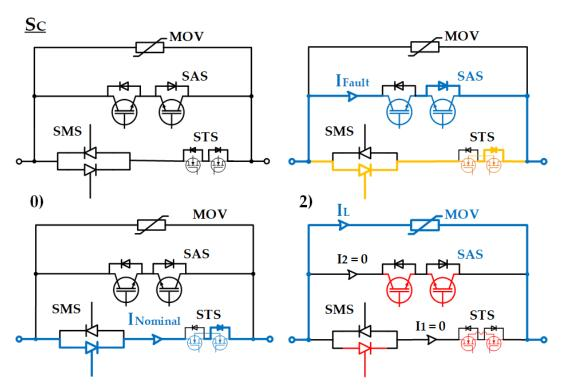
**Figure 1.9:** 0) Normal condition: SMS and STS in conduction; 1) STS turning off: fading current (yellow line) in main branch; 2) Note that SAS must be turned off only after the thyristor is blocking (I1=0 and then I2=0); MOV: Metal Oxide Varistor, SAS: Semiconductor Accessary Switch, STS: Semiconductor Transfer Switch
