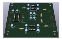
Figure 5.5: Design of the IGBT driver board
