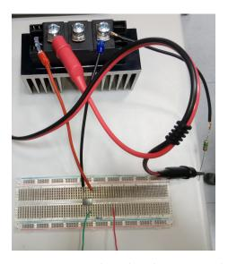
Figure 5.4: SCR gate driver based on optocoupler
