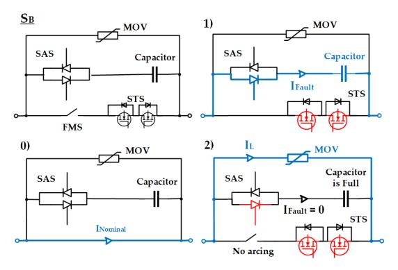
**Figure 1.8:** 0) Normal condition: FMS is closed; 1) Fault condition: a fault signal switches off the STS what commutates the fault current to the thyristor branch; 2) The same fault signal opens (with the corresponding delay) the FMS. Meanwhile, the thyristor started blocking once the capacitor became fully charged; MOV: Metal Oxide Varistor, SAS: Semiconductor Accessary Switch, FMS: Fast Mechanical Switch, STS: Semiconductor Transfer Switch
