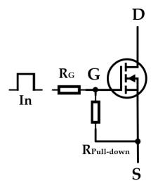
**Figure 3.7:** Essential gate driver circuit to drive a voltage controlled switch.  $V_{IN}$ : voltage provided by the gate driver.  $R_G$ : gate resistor.  $R_{PD}$ : gate pull-down resistor [34].
