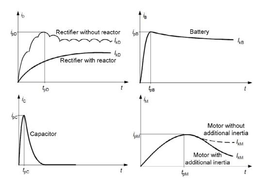
Figure 3.1: Short-circuit waveforms for a) rectifier, b) battery, c) capacitor, d) motor [16].
