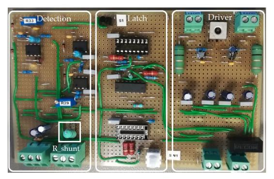
Figure 5.1: Detection board
