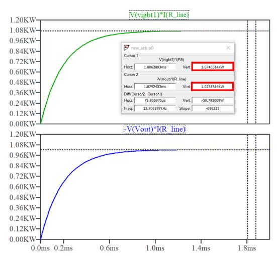
Figure 4.7: Steady-state power loss if the IGBTs stay conducting
