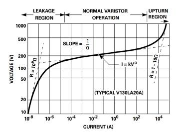
Figure 3.15: V-I characteristics in three regions, plotted in log-log scale [19]
