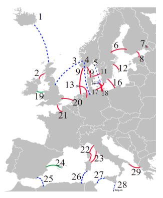
Figure 1.5: HVDC links. Red: existing, Green: under construction, Blue: planned. [31]
