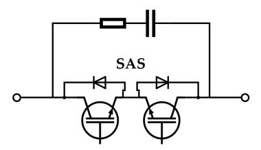
Figure 6.2: Power circuit of the IGBT Breaker
