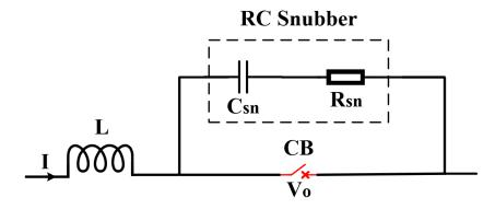
Figure 3.14: Unidirectional solid state circuit breaker
