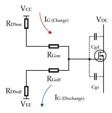
Figure 3.9: Gate currents for charging and discharging modes [20].
