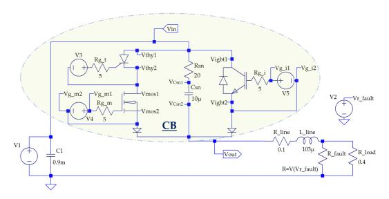
Figure 4.1: Single-phase microgrid circuit. Modern circuit breaker inside the oval
