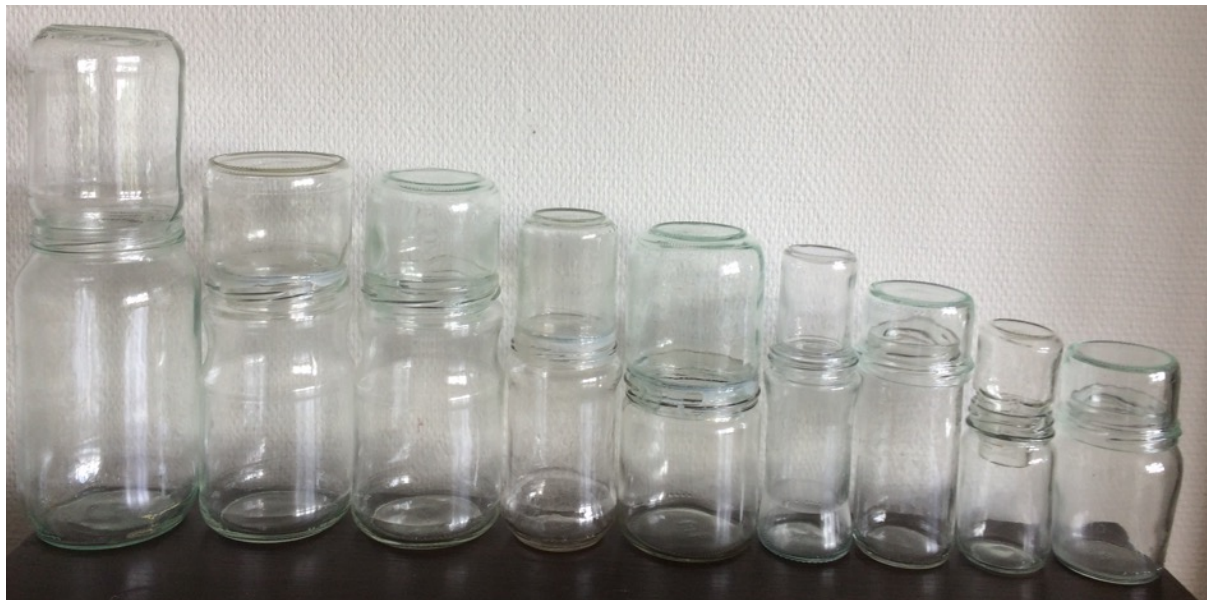
Figure 7: These many different jar-bricks are made of 2 jars with similar diameter and tops fit nicely together; notice here that one has an exterior and interior surface, but only one air chamber.
