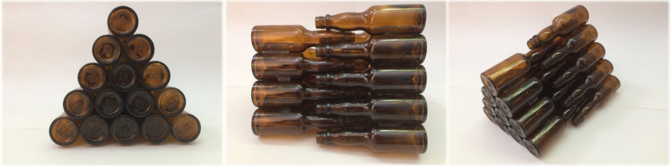
Figure 3.1: Front view, side view and perspective view of Licorice-bottle DSF system without the in-fill
