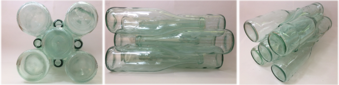
Figure 3.3: Front view, side view and perspective view of Wine-bottle DSF system without the in-fill
