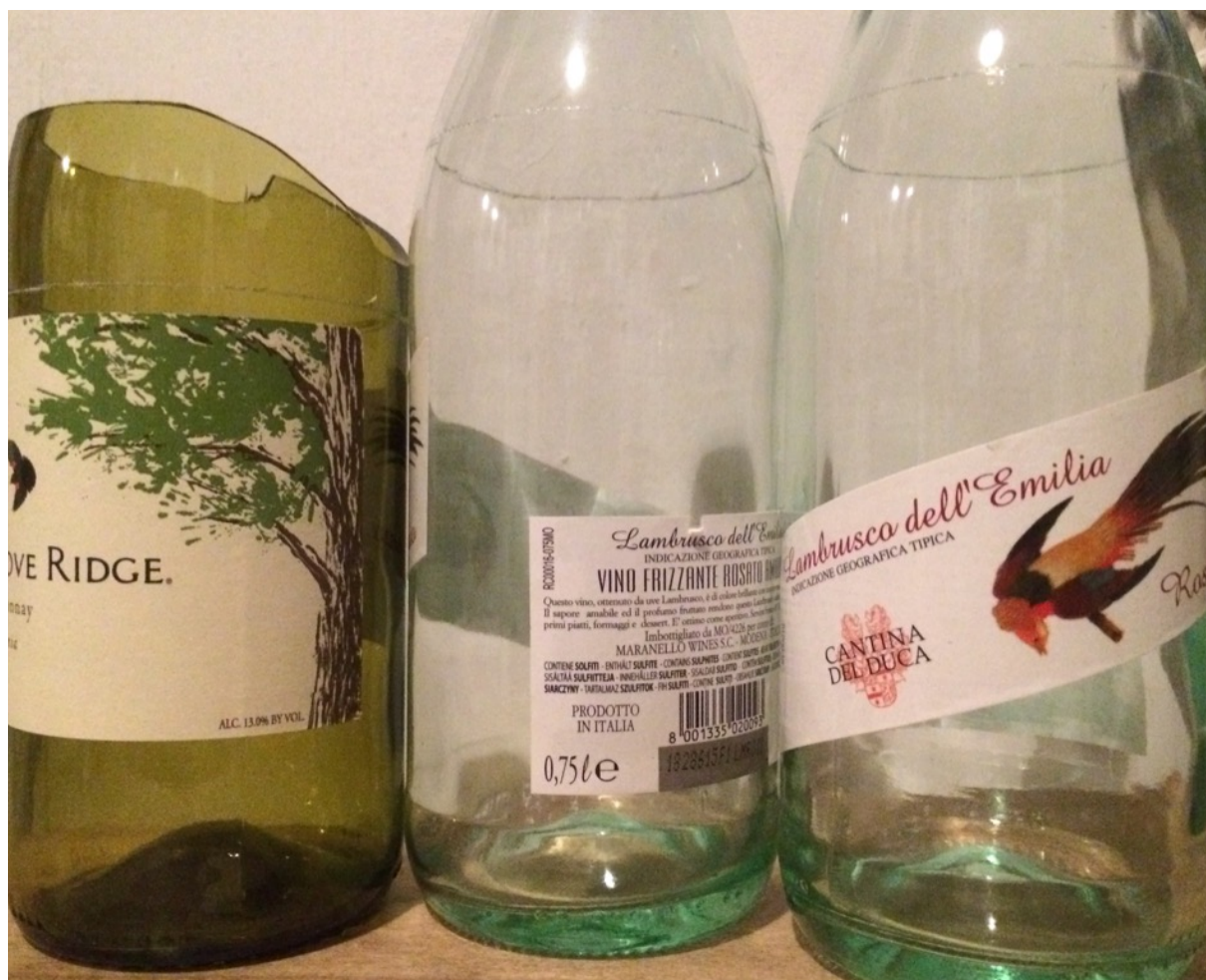
Figure 8: My first efforts proved no good — the bottle on the left broke no where near the scored line.
