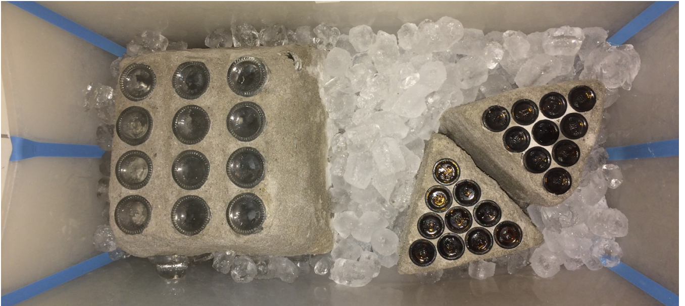
Figure C.2: Prototypes are placed in container with ice cubes around them to reduce thermal influence from indoor environment.
