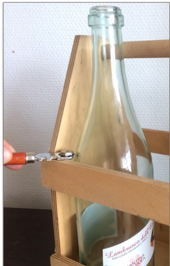
Figure 4: Bottle is placed in a toolbox which acts as a jig — coincidentally this height proved to be ideal due to the curve of the neck of the bottle.
