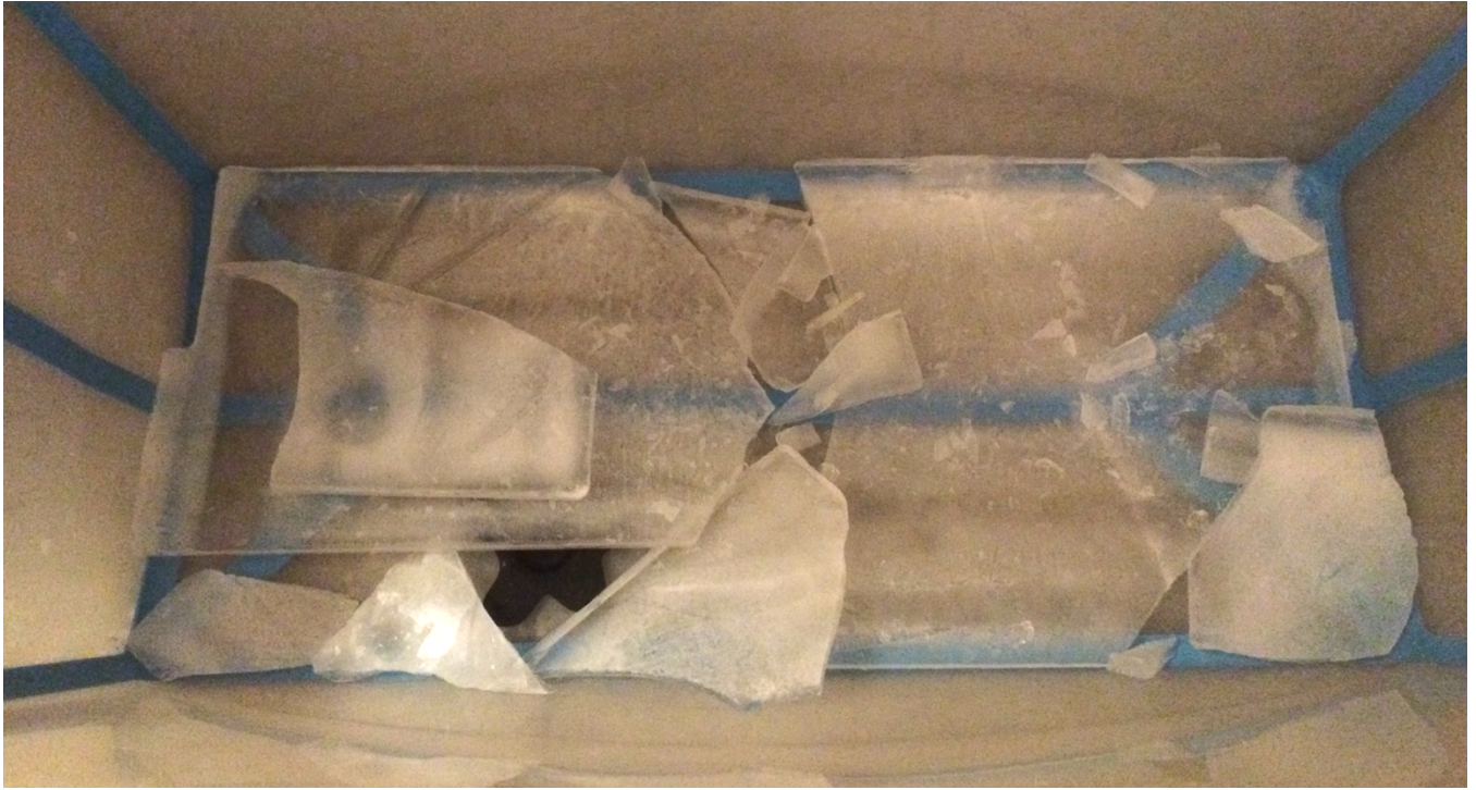
Figure C.1: A flat layer of ice does not cover completely the surface of the container but that is of little significance since the prototypes are on each ice sheet and gets consistent cooling.
