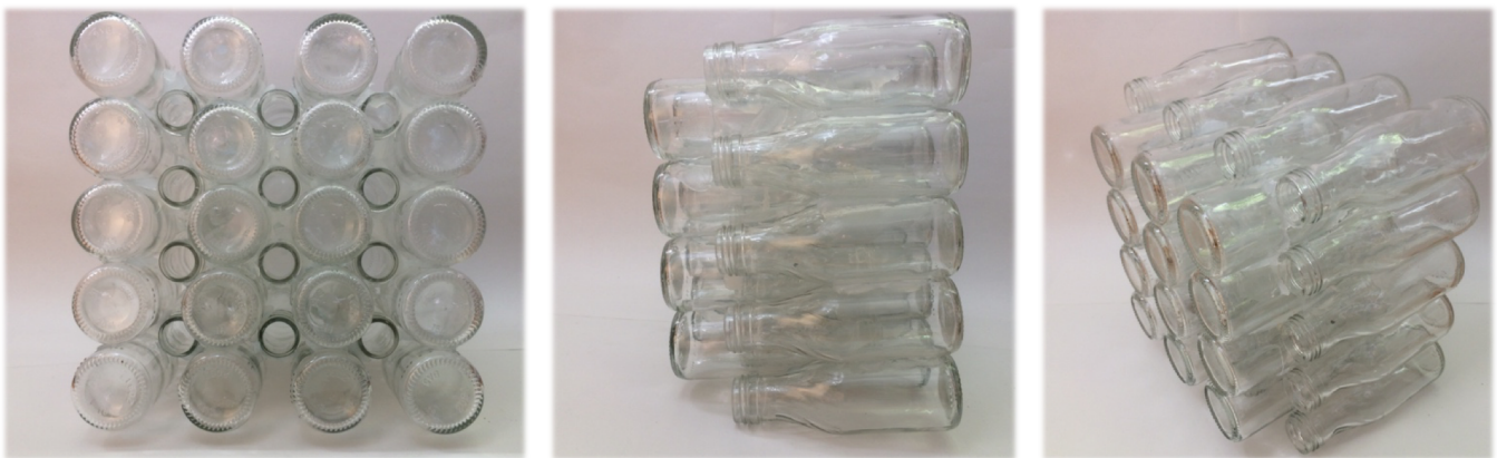
Figure 3.2: Front view, side view and perspective view of Creamer-bottle DSF system without the in-fill
