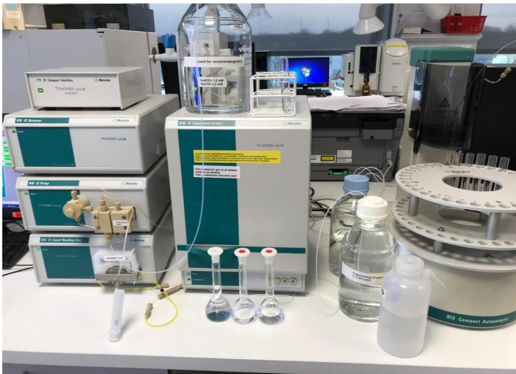
Figure 4.2-1- Ion Chromatography (IC) machine
