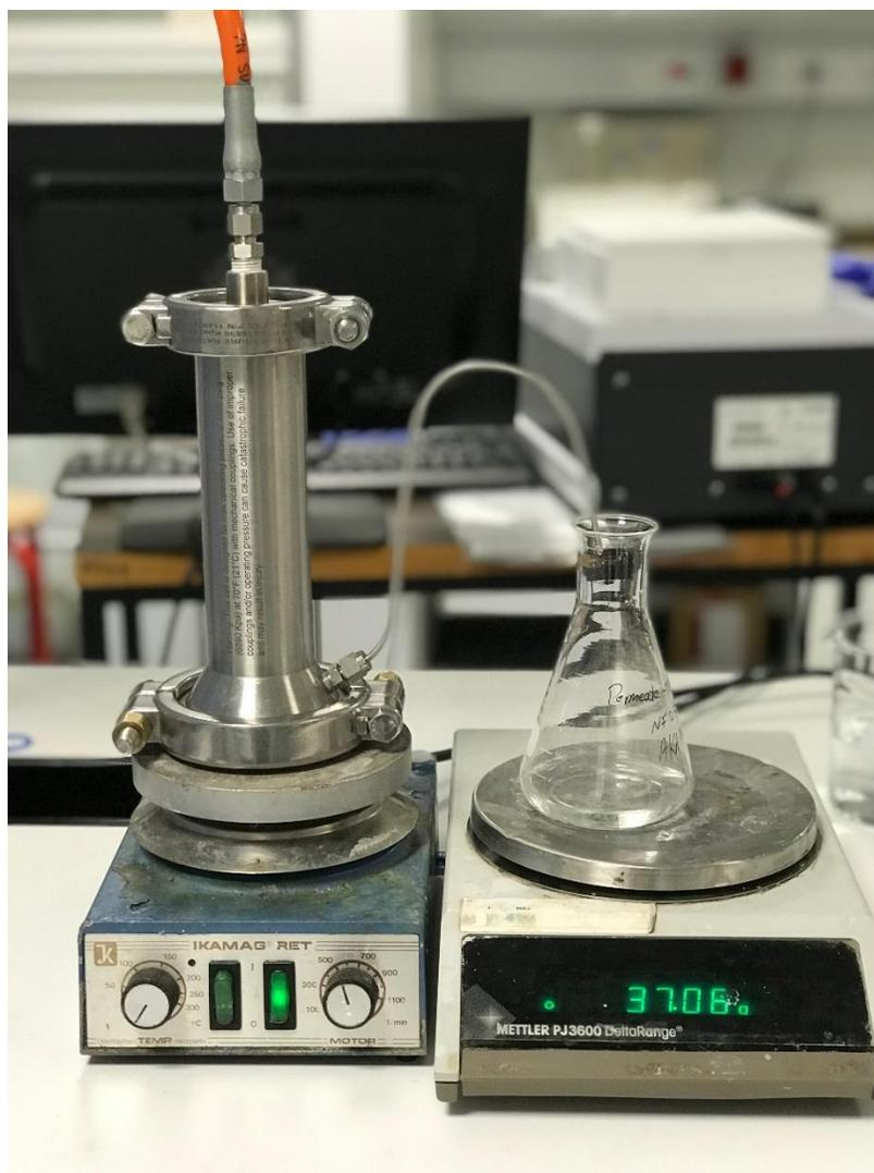
Figure 4.2-6- Dead-End Process, experimental setup for both nanofiltration and reverse osmosis membranes experiments
