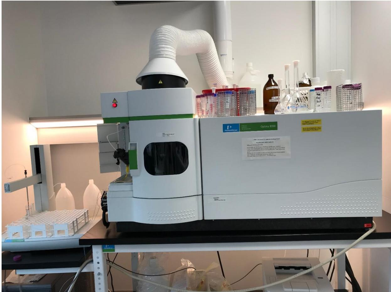
Figure 4.2-2- Inductively Coupled Plasma-Mass Spectrometry (ICP-MS) machine
