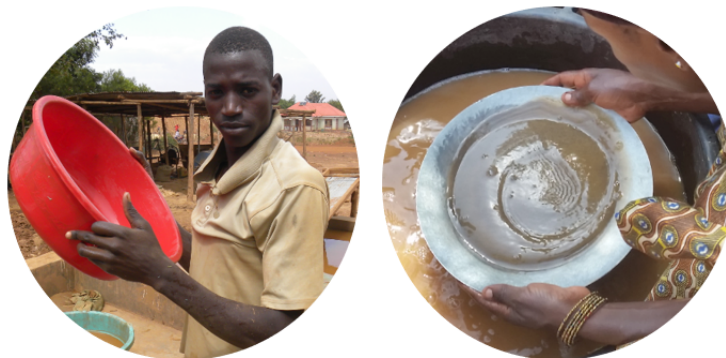
Figure 17. Comparison between the traditional African pan and "ninja" pan used by the trainers from the Philippines.
