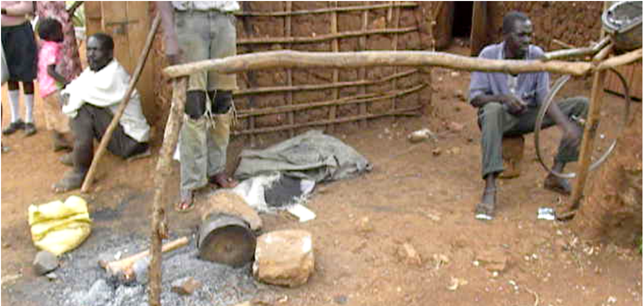
Picture 1: Artisanal arrangement for a manual blower, built with scrap metal elements, a wheel from a bike and a rope.
