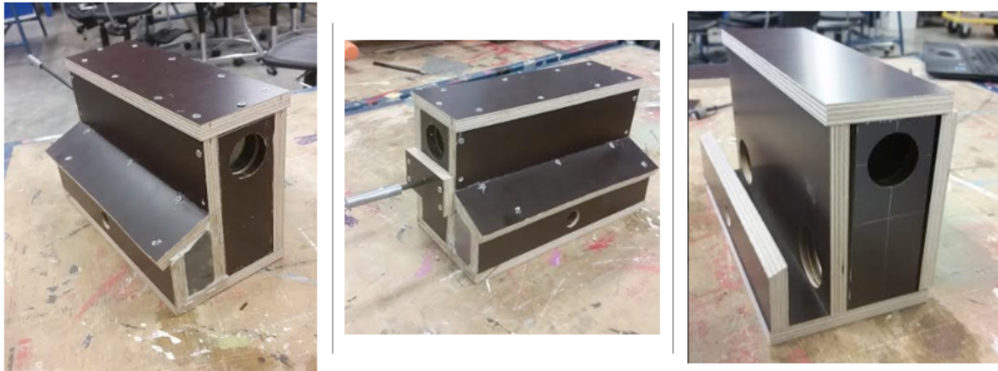
Figure 6. The prototype of a Japanese blower “Fuigo” as a mechanism to be used in the workshop with the miners.
