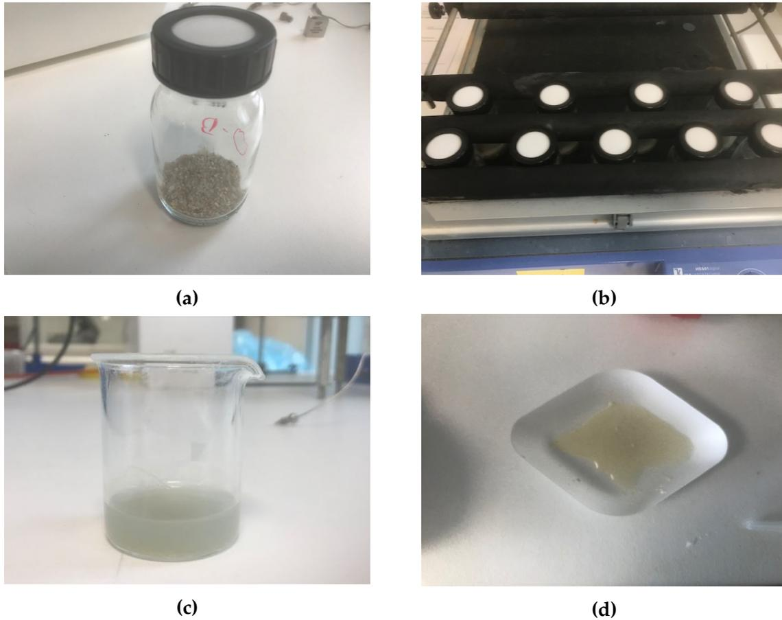
**Figure 4.5:** Experimental setup used in the soil slurry experiments showing (a): Glass bottle used as a model batch reactor (b): Shaker plate setup (c): Catalyst + OA mixture (d): CP slurry
