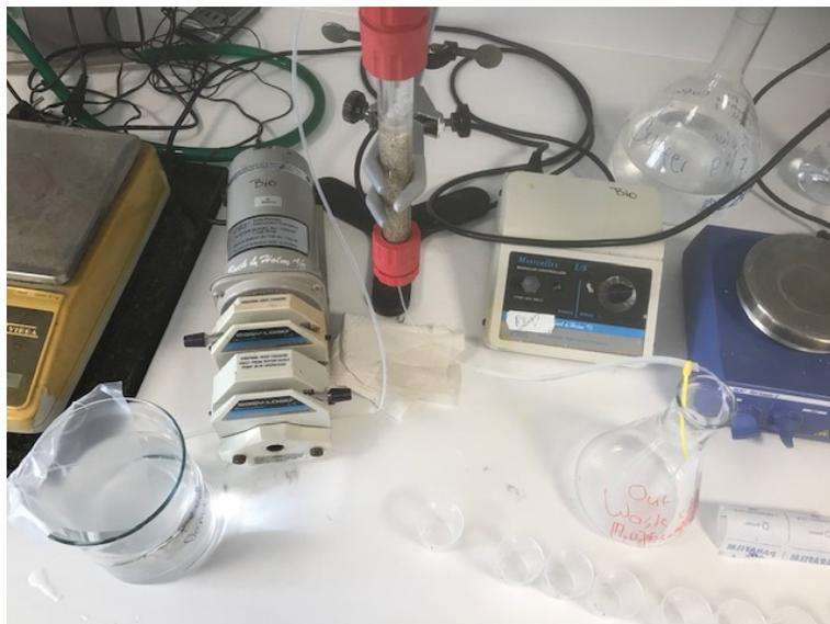
**Figure 4.6:** Illustration of the column set-up used with pump (left), column
