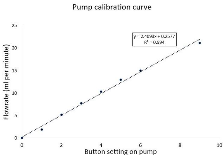
Figure 8.2: Calibration curve for the pump used in the column studies.
