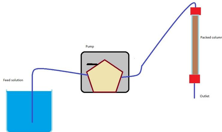
**Figure 3.1:** Schematic illustration of the column set-up consisting of feed solution (left), pump (middle) and column (right).
