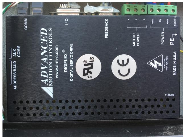
**Figure 3.3:** One of the four AMC DPCANTR-040B080 motor drives, situated in the robot, one for each motor. Seen from the top left to right is the CAN-bus connection, followed by the input/output port. Next comes the feedback port, followed by the power connection, both connected to the motor. Finally the power input to the drive is seen, which is split in high power to the bridge and logic power. On the left side the auxiliary port for communication with the drive is seen.
