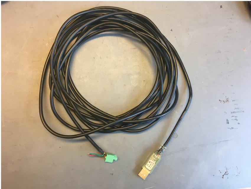
**Figure A.1:** When using DriveWare, it is necessary to connect to the auxiliary port on the drive. Use a USB-RS232 cable with a Phoenix 1881338 plug mounted. Remember to turn on the drive!
