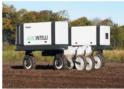
(b) The field robot "Robotti", developed by the Danish company Agrobot.[1]
