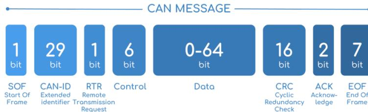
**Figure 4.1:** A representation of a CAN message. Note that this particular message is the 2.0-B extended version with the 29 bit identifier.
