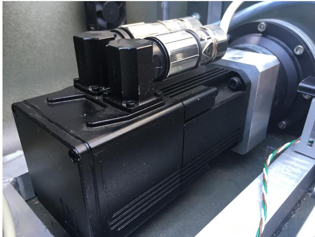
**Figure 3.4:** One of the four A/C servo motors situated in the robot. A gearbox is mounted on the motor and each wheel is then mounted on the end of the gear shaft. There is two cables connected to the motor, one for power and one for the feedback signal to the drive.
