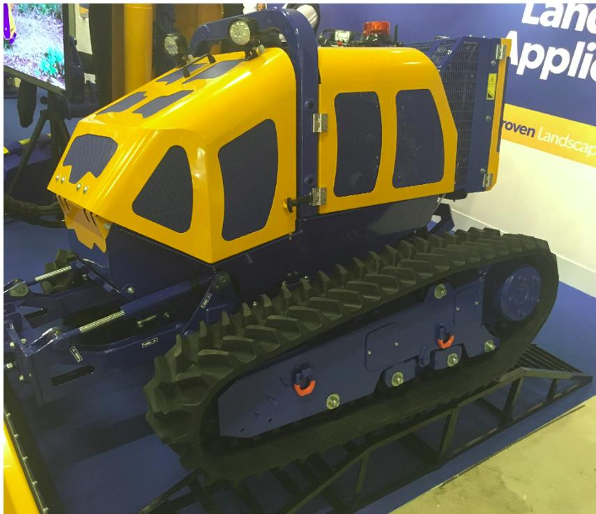
**Figure 2.3:** A conceptual representation of a field robot, equipped with tracks. This specific machine is not designed for autonomous use, but is remotely controlled by the user. Weight 1,200 kg. [6]
