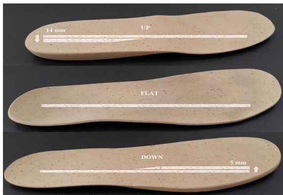
Figure 2: Custom insoles with 14 mm heel spring ("UP"), flat ("FLAT"), and 5 mm forefoot elevation ("DOWN") [27].
