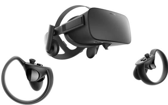
**(a)** The Oculus Rift head mounted display and controllers.
