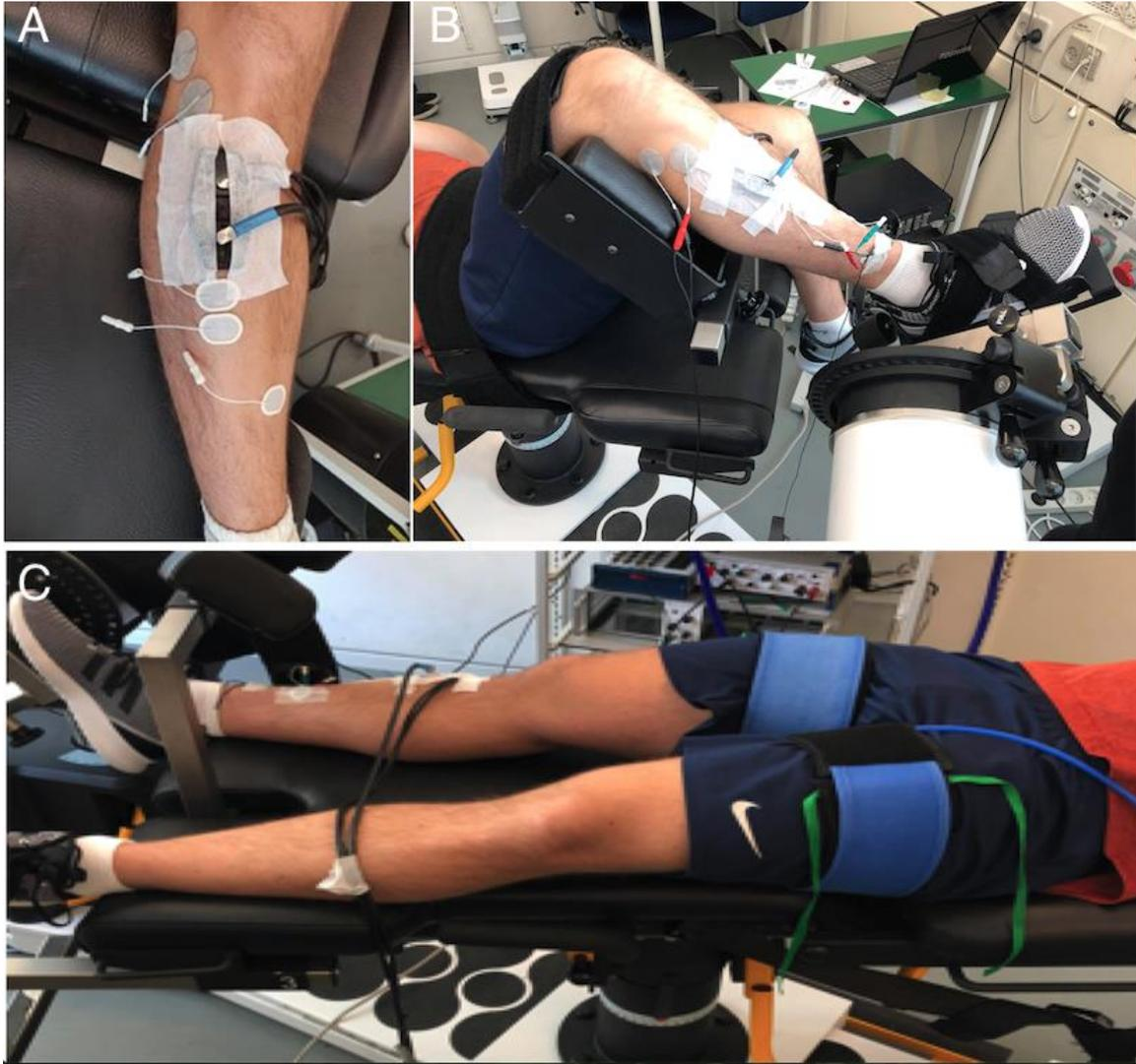
Figure 2: A) The placement of surface EMG electrodes, NIRS apparatus and stimulation electrodes. B) Experimental setup in the dynamometer. C) Cuff placement during IPC/sham protocol.
