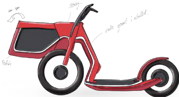
Figure 02.24. This concept can be used as a scooter in standing position and as a scooter in seated position as it has a retractable seat integrated. The tools etc. are stored in the front and the cargo hold in the front can be tilted for offloading.
