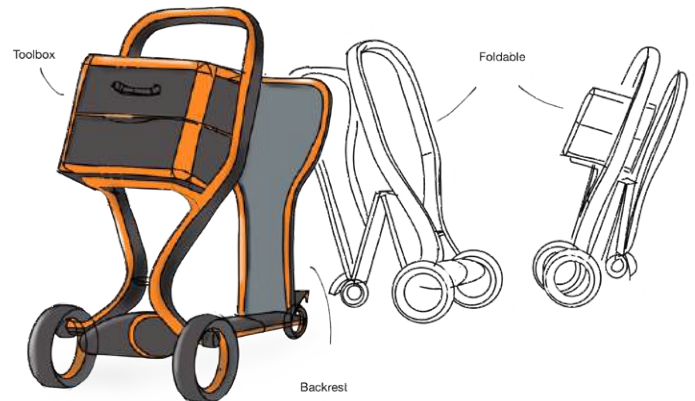
Figure 02.1. A small foldable e-scooter with storage room for tools. The scooter has a backrest instead of a seat to provide support.
