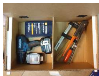
Figure 03.8. Testing if the basic tools are able to fit into the “basic toolbox”. The handle in the middle works as a smaller divider of the tools. Underneath the “basic toolbox”, the “extended basic toolbox” is placed. This should be able to store some of the larger tools the PMTs use. The two toolboxes with different tools. Having two toolboxes in one provides a better overview of the tools the PMT brings. The “extended basic toolbox” has a divider which can be used to separate the tools. The divider can be placed as the PMT prefers.
