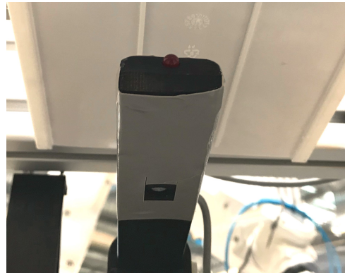
Figure 6.9: Sensor Stick Containing LED and Motion Sensor
