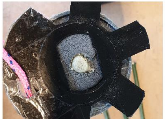
Showing the end of the cable reel. This act as a brake which provent all of the rope to fall of at once. .
