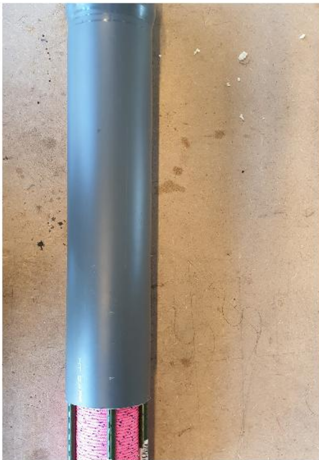
Showing the outer PVC tube which is acting as a protecting shell..
