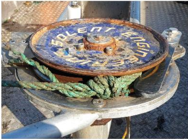
The hauling tool is hauling in the first creel and a knot can easily go through it. This means that our attachment
