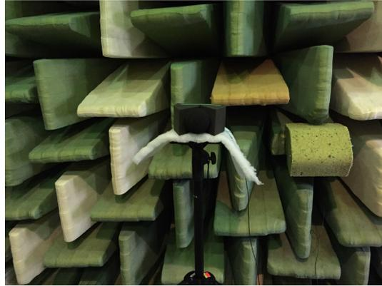
**Figure D.7:** The picture shows the measurement microphone with the large foam wedge configuration two
