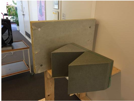
**Figure E.14:** The picture shows the measurement with the large wedge and single rockwool bat, configuration five.
