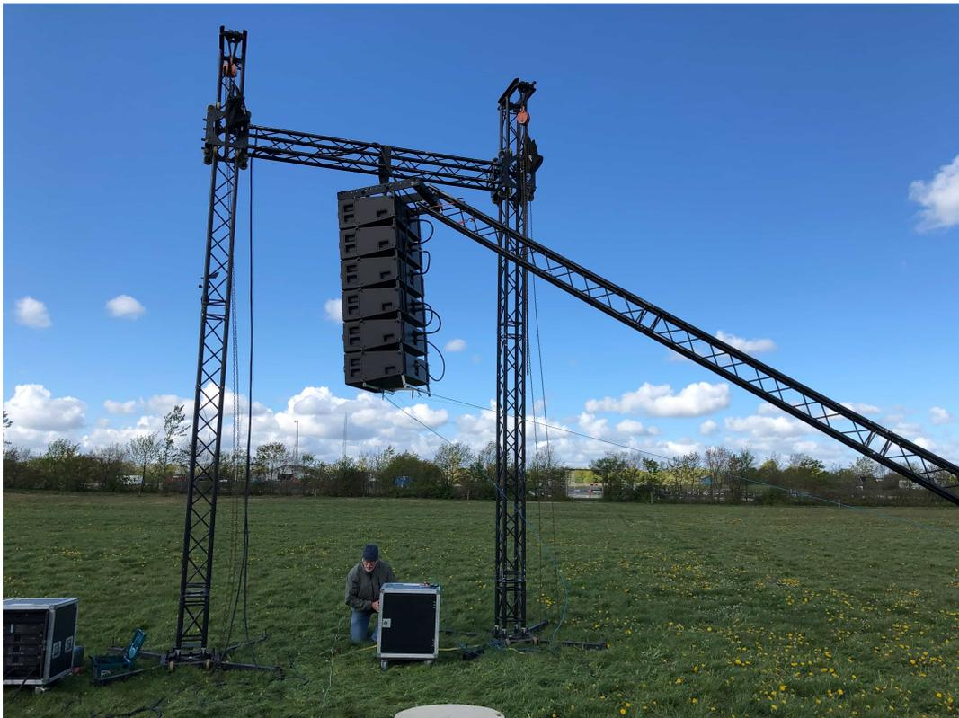
**Figure 9.1:** The picture shows the measuring setup while the parallel wind measuring is under preparation.
