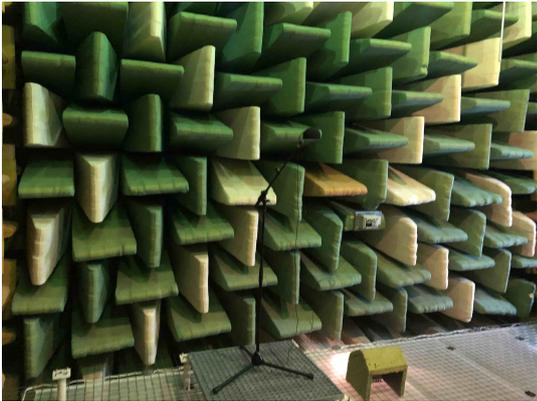
**Figure M.3:** The picture shows the measurement microphone with the original modified windscreen.
