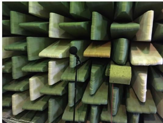
**Figure D.4:** The picture shows the measurement microphone with the original windscreen
