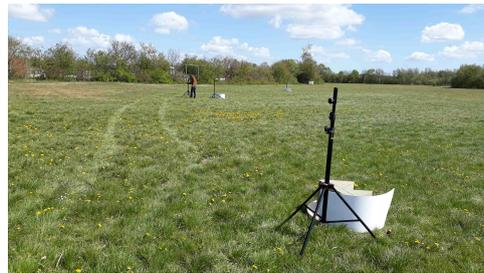
(b) The figure shows the microphone setup for crosswind
