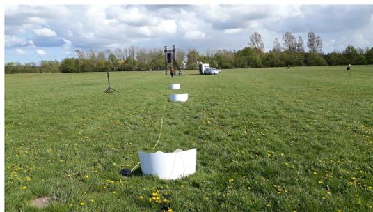
**Figure P.4:** The figure shows the microphone setup for parallel wind condition.
