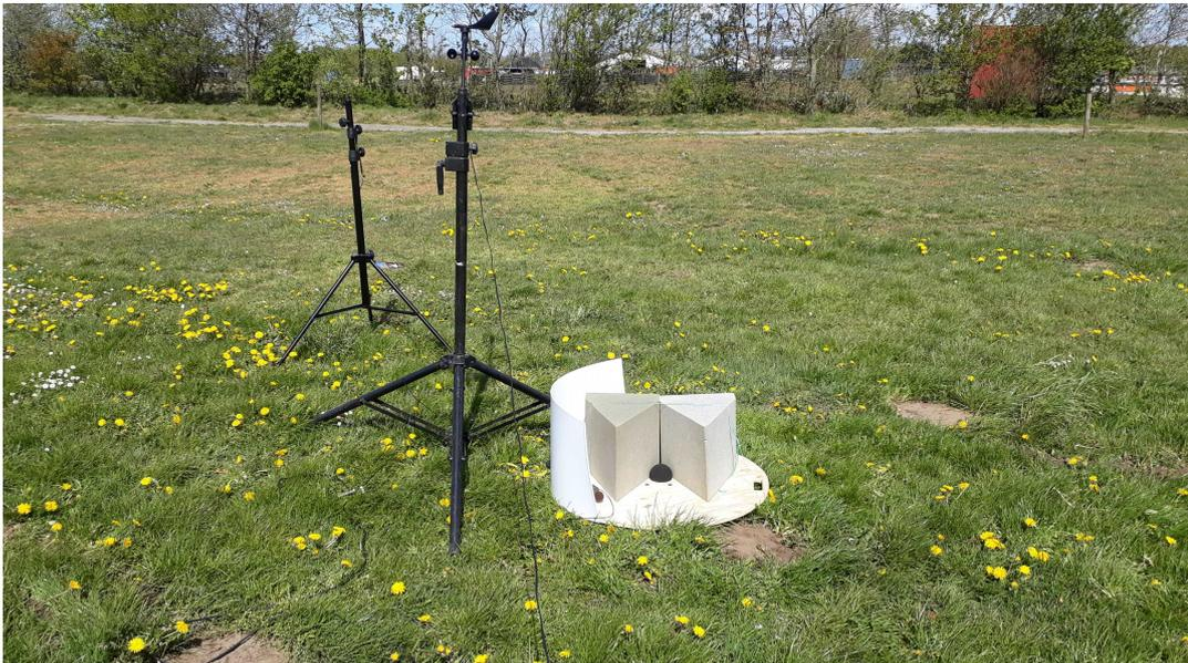
**Figure 7.18:** The picture shows the designed windscreen while it is prepared for crosswind measurement.
