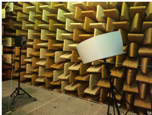
**Figure M.10:** The picture shows the measurement microphone with the tilted designed windscreen.
