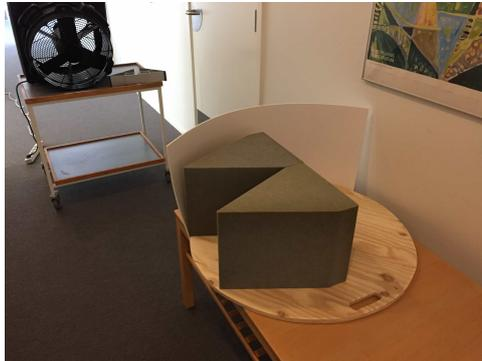
(a) The picture shows the measurement setup for the optimised windscreen configuration five from back
