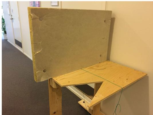
**Figure E.11:** The picture shows the measurement setup for the single rockwool bat, configuration four
