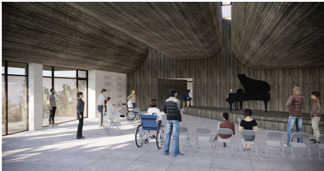
Figure 7.3.27: The design of convex roof has the purpose to diffuse the sound of music to the audience
