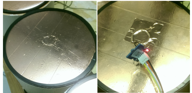
Figure 2: The Grove sensor attached to the underside of an acrylic glass surface, on copper tape.
