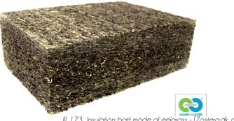
III. 173 Insulation batt made of eelarass - [Zostera.dk, n.d.]
