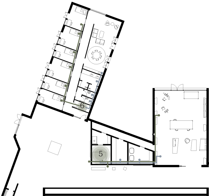
Ill. 6.14 ventilation principle - aggregate 5+6 (atelier and artist rooms )
