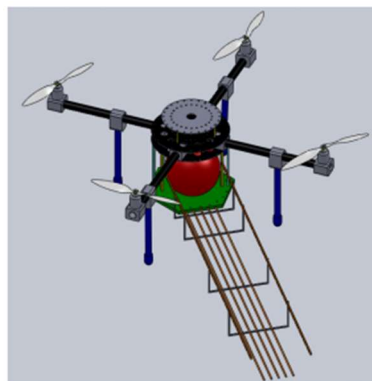
Figure 6.6 - Quadcopter with cage and railing system designed by [41]
