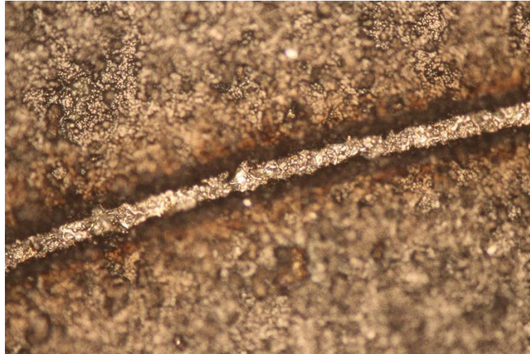
Figure 10: Example for laser ablated circle line of which the entire coating was removed and stainless steel is exposed. Picture was taken with 50 fold magnification.
