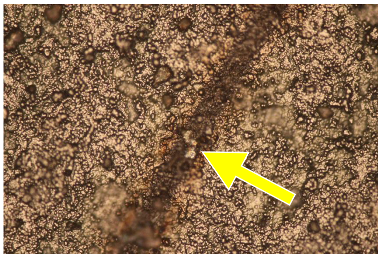
Figure 11: Example for laser ablated circle line which shows small defects. The defect, where stainless steel is exposed, is shown by an arrow. Picture was taken with 50 fold magnification.
