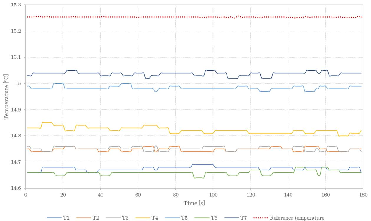
**Figure C.11:** Sensirion temperature comparison with reference thermometer at 15 °C
