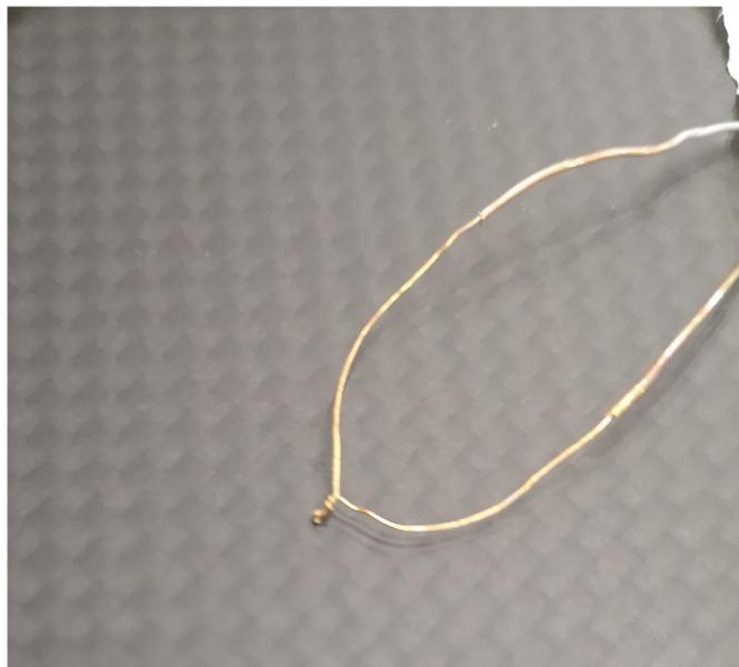
The golden coating has come off on one of the thermocouples.
