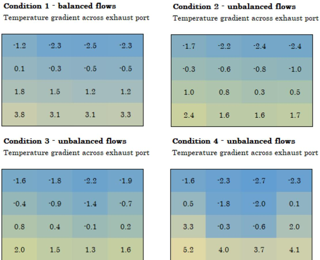
**Figure 7.6:** Temperature gradient on exhaust port for all test conditions
