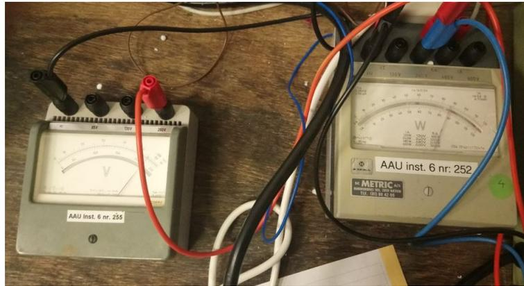
**Figure A.1:** Voltmeter and watt meter to measure power consumption
