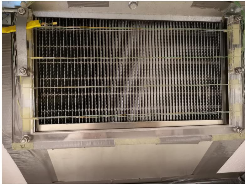
**Figure 5.4:** Thermocouple grid placed on the heat exchanger
