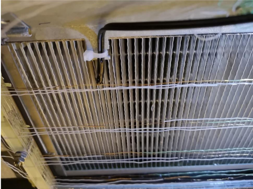
**Figure E.8:** Bigger droplets of condensation at second 3000 - condition 2
