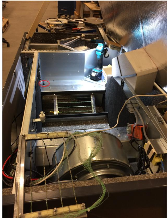
**Figure 5.8:** Pressure tap on the extraction side
