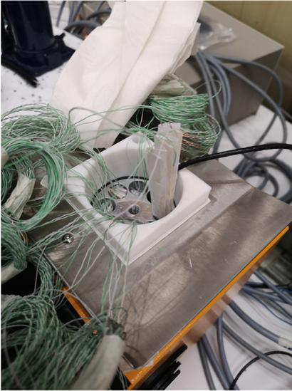
Thermocouples folded and taped form one side on the paper to avoid short circuit. The tip (measuring point) is not taped.
