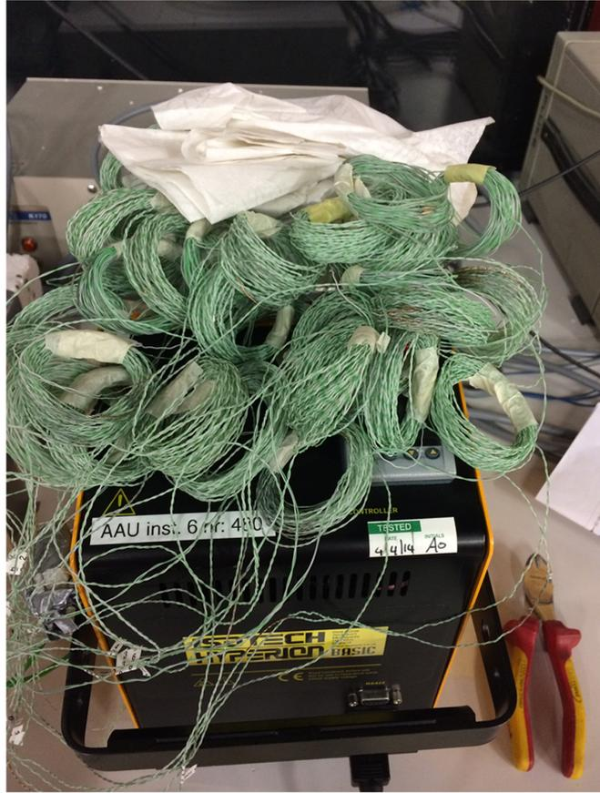
Thermocouples inside the Isotech box during calibration process.
