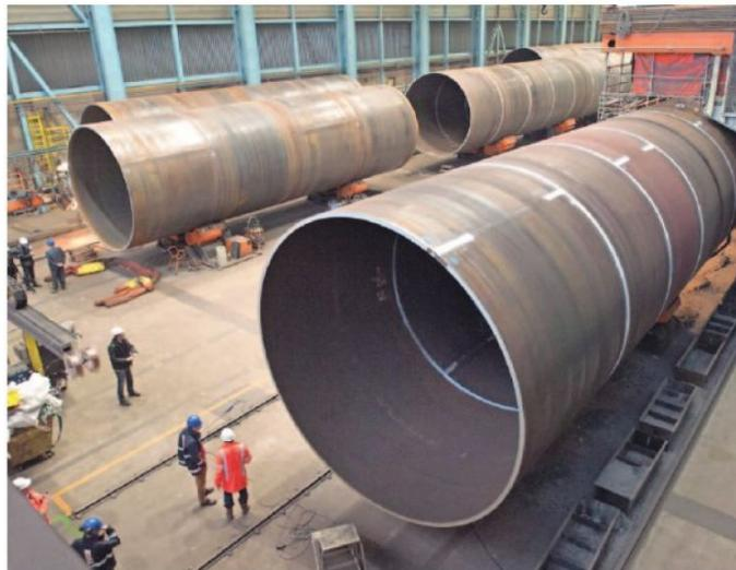
*Figure 1.2.* Monopile sections welded together [Krabbendam, 4 January 2017]
