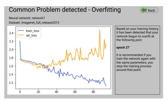
Figure 4.5: A sketch of the menu describing common problems with neural networks in the application. As an example, this sketch shows a case when the neural network started overfitting.
