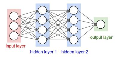
Figure 2.1: An example of a feed forward neural network [8].
