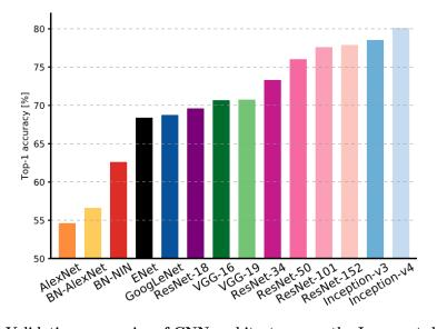
Figure 2.7: Validation accuracies of CNN architectures on the Imagenet dataset [16].
