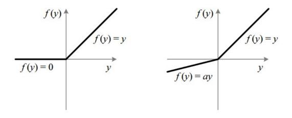
Figure 2.15: The Rectified Linear Unit Activation Function (on the left) as compared to the Leaky Rectified Linear Unit Activation Function (on the right) [9]
