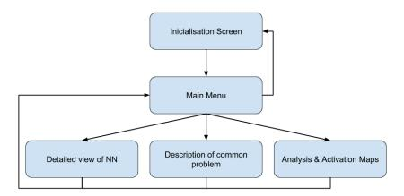
Figure 4.1: Flowchart, showing how the menus of the application connect to each other
