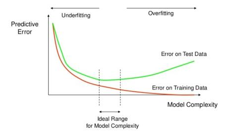
Figure 2.4: If the neural network is trained for too long it loses its ability to generalise and starts to overfit based on the training data. Because of this, there is an ideal time range when the taining should be stopped [13].
