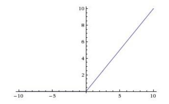
Figure 2.14: The Rectified Linear Unit Activation Function [25].
