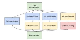
Figure 2.10: An inception module of the GoogleNet, where three seperate convolutions and one pooling is parallelized in a single module. Notice how a 3x3 convolution is preceded by a 1x1 "bottleneck" convolution, and the 3x3 pooling is followed by an additional 1x1 "bottleneck" convolution to reduce the dimensionality of the output filter [19].
