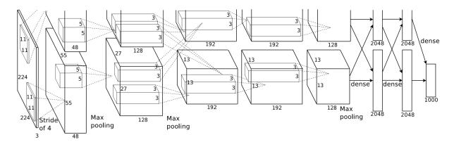
Figure 2.9: Architecture of the AlexNet, starting with a convolutional layer, leading to a pooling layer, leading to normalisation, then leading to another convolutional, normalisation and then a number of convolutional layers, finishing with a pooling layer and then three fully connected layers. The picture in the original paper is missing its top part, and is cited as such in academic sources as well [17].
