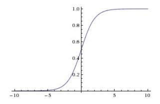
Figure 2.12: Sigmoid non-linearity function, normalizing real numbers to range between 0 and 1 [8].
