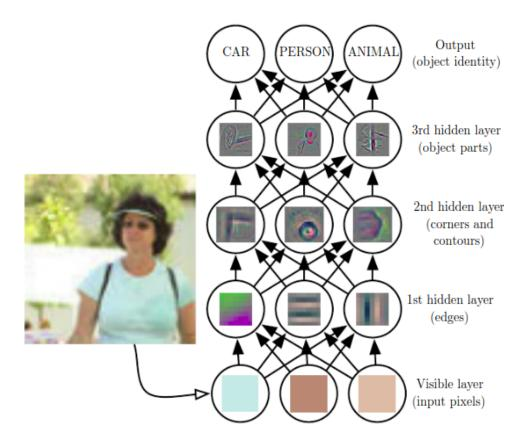
Figure 2.5: Convolutional networks follow the same principle as regular neural network, with the pixels of the picture being the input, the network learning more general and high level principles in its earlier layers, getting more and more specialised in the deeper layers, and returning a classification in the output layer [14].
