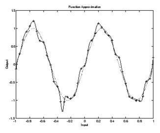
Figure 2.23: A 1-20-1 neural network attempting to approximate the underlying sine wave. The dotted line shows the underlying sine function, the noisy measurements are marked by + symbols an the response of the neural network is marked as the solid line [39].
