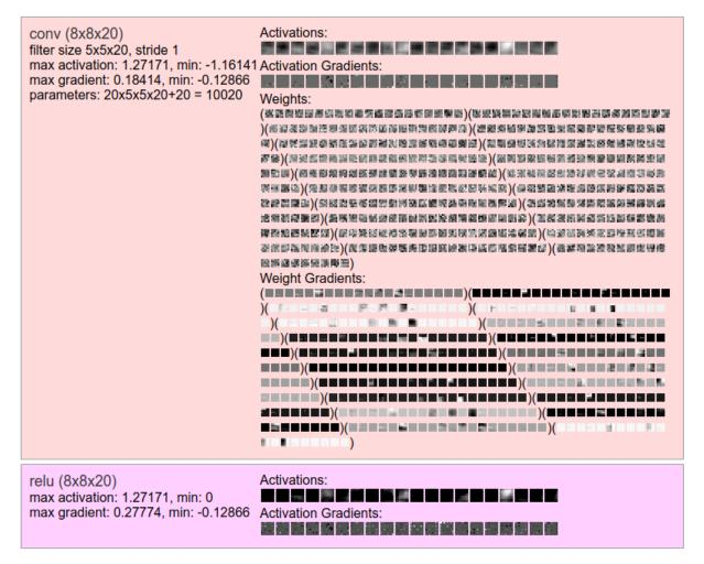
Figure 2.21: An example of the filters learned by the third convolutional layer of a neural network, trained on the CIFAR-10 dataset and ran through the visualisational demo of Stanford University at [36]. The input image is the same ship as on Figure 2.20
