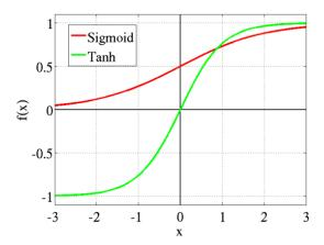
Figure 2.13: A comparison between the Tanh and the Sigmoid functions [9]
