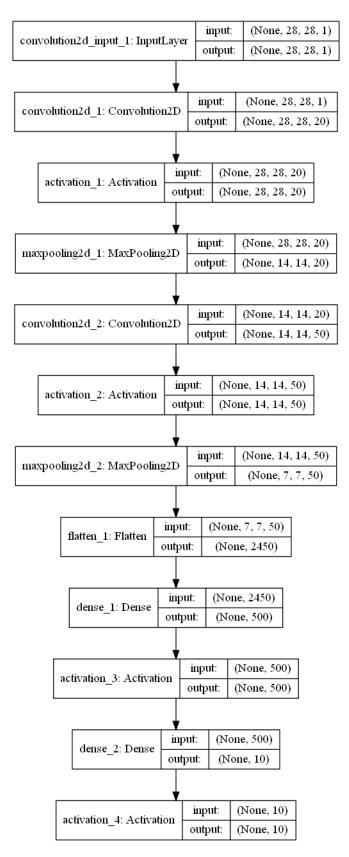
Figure 2.19: The model summary as provided in Keras with the keras.utils.vis\_utils function. This image contains information about each layer's role, their output shape and their number of parameters [35].
