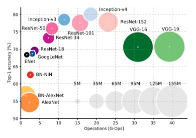
Figure 2.8: Chart showing the operations required for a single forward pass with the network (on the x-axis) in comparison to the classification accuracy of each model (y-axis). The size of each disk is proportional to the size of the neural net produced [16].
