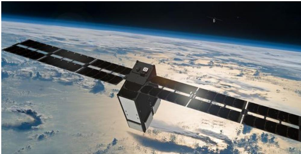
Figure 1.1: Nano-satellite with deployable solar panels [\[3\]](#)
