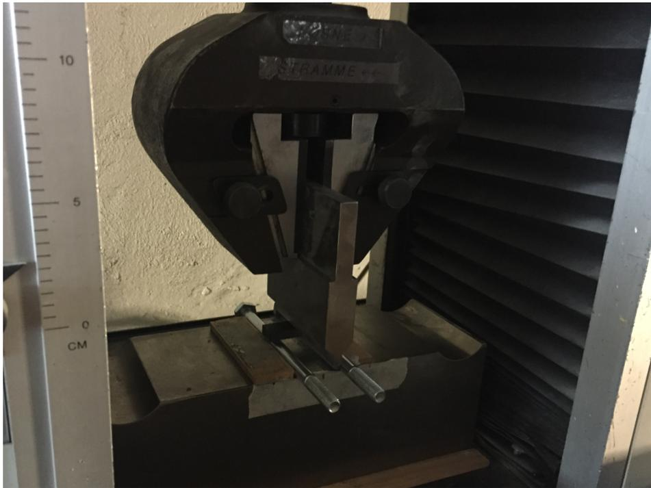
Figure 4.1. ILSS test set-up.
