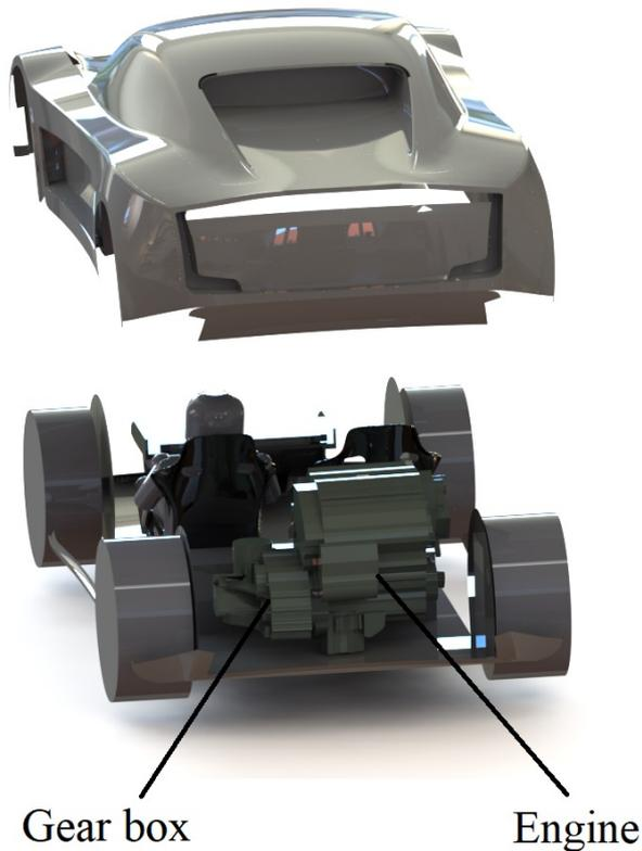
*Figure 2.2.* Car components. View 2.
