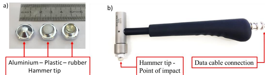
Figure 9-1: Impulse excitation equipment. a) Three hammer tips with different hardness. b) Brüel & Kjær Impact Hammer Type 8206 [21].
