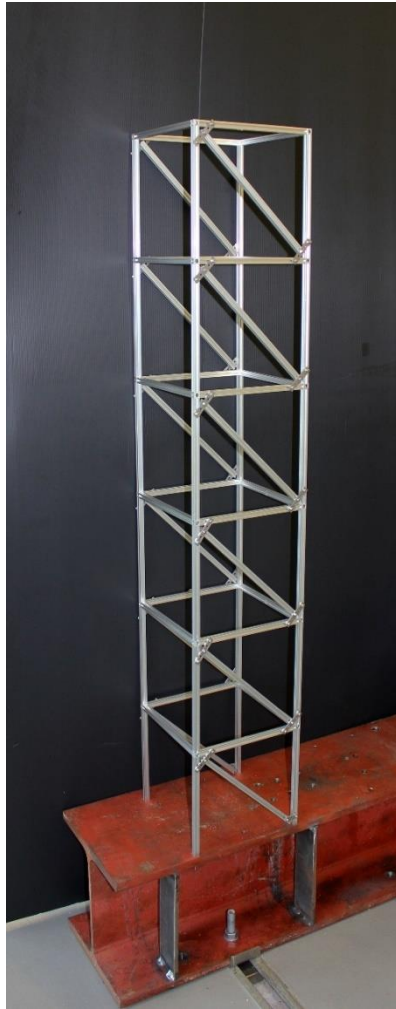
Figure 1-3: Frame structure on top of I-profile used for fixation.
