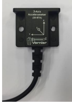
Figure 9-4: 3-axis accelerometer model “LoggerLite 3D-BTA”.
