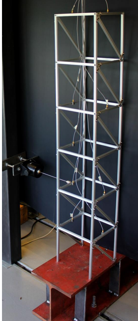
Figure 3-8: Experimental setup of frame structure.
