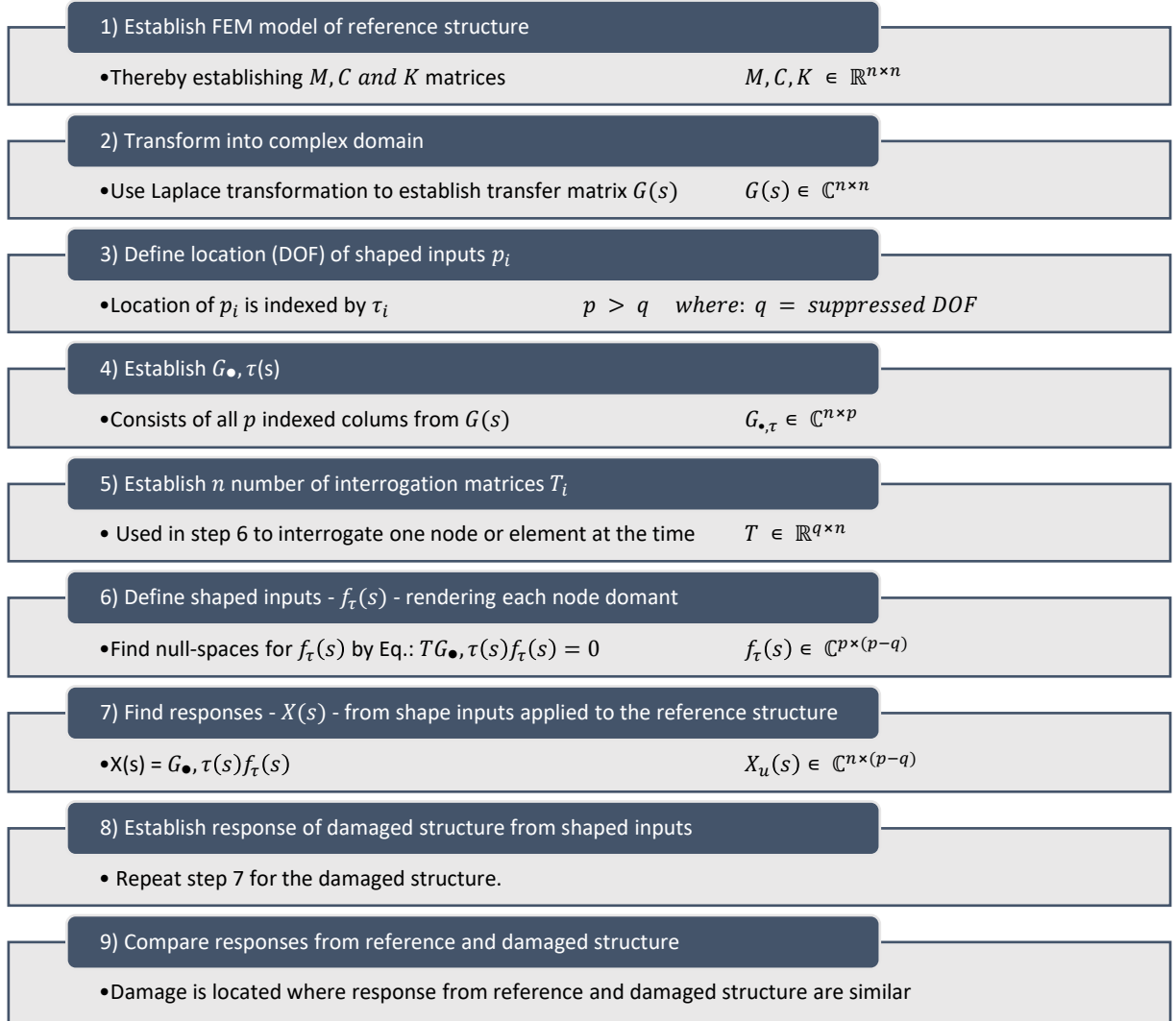
Figure 2-15: Flow diagram for localisation of damage using SDLID.
