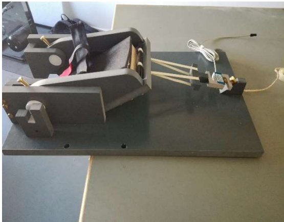
Figure 1 Mounted ergometer, with the force transducer installed. It can be seen the place in which the potentiometer will be inserted.
