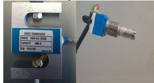
Figure 3: On the left, the force transducer; on the right, the potentiometer with the layer of tape, which was necessary to assess a perfect adhesion to the rotating pin.
