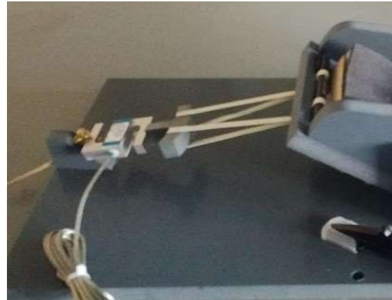
Figure 2: detail of the connection between the force transducer; from left to right it can be seen the inelastic rope, the plastic connecting part, the transducer, the t-shaped element and the elastic bands, connected to the foot plate.
