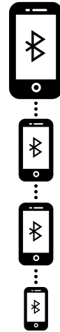
Figure 4: The largest phone is the master, the two medium size phones are master slaves, the smallest device is a slave and together they form a scatternet consisting of three piconets.
