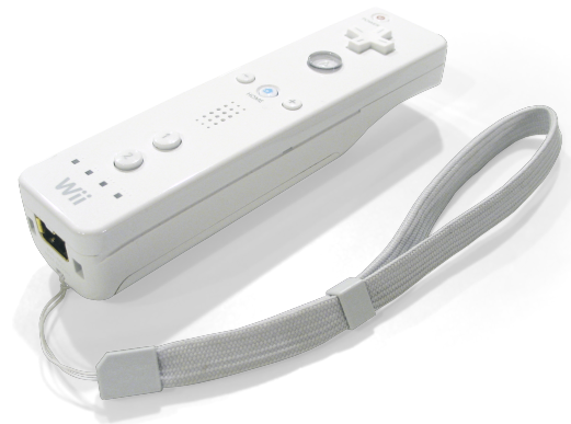
Figure 2.6: Nintendo Wii Remote; With accelerometer to register movement, as well as a sensor placed near the TV that allows the remote to function as a pointer ( Wii Remote , 2018).
