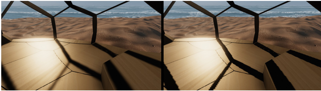
Figure 5.6: Soft shadows turned on (left) and hard shadows turned on (right), where the hard shadows have more jagged edges and the soft shadows look smoother.
