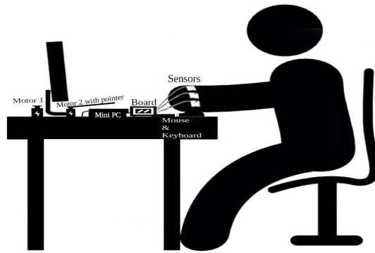
Figure 17. The experiment set up. The user uses a keyboard and a mouse to set the connections between the sensors, the motors and the visual on the computer screen.
