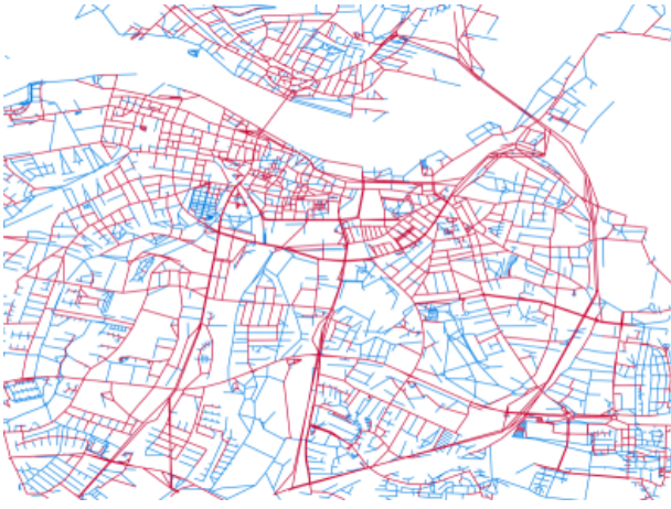
Fig. 6: Aalborg network. The red segments have been rendered thanks to the trajectory GPS data. For these segments exists enough information to derived travel cost distribution. For the blue segments the speed limits have been used to derive travel cost. [1]
