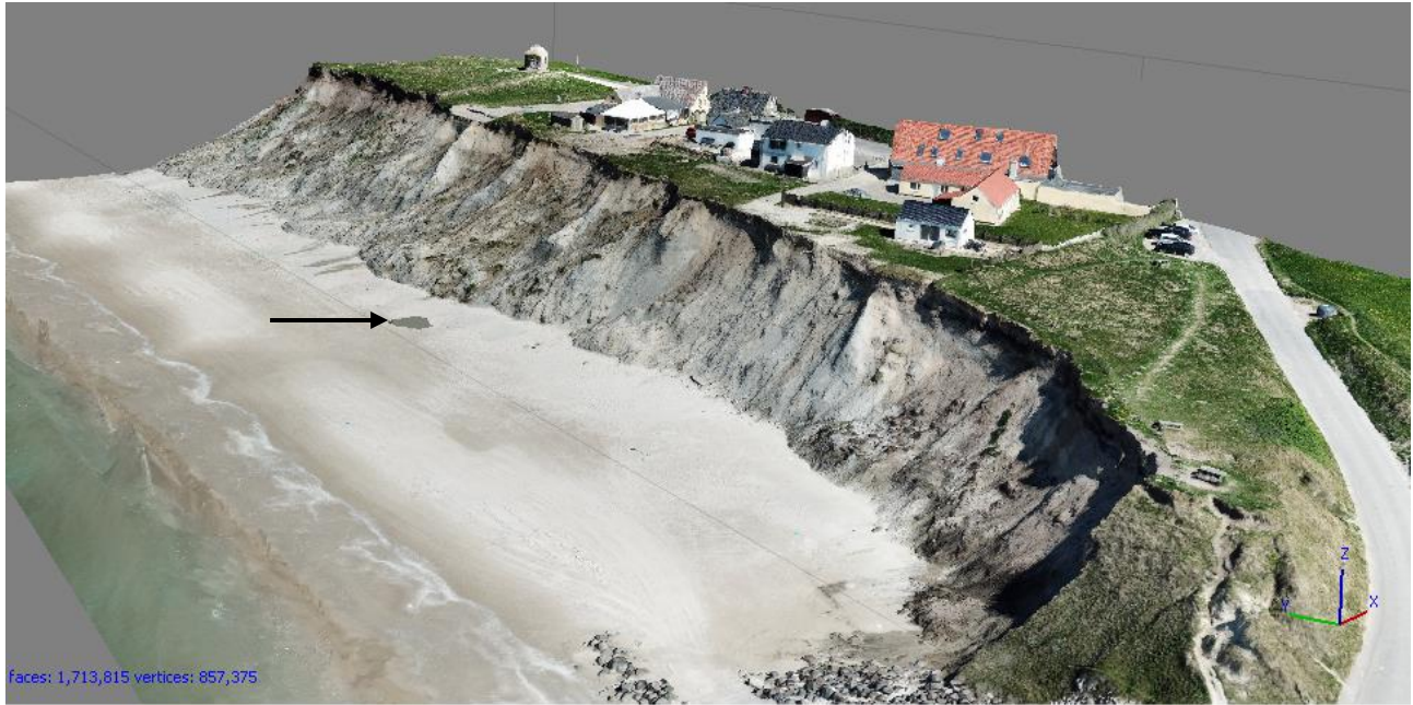
Figure 6.2 - Exported image of the 3D model constructed from images acquired on the 14 th of May 2018. The black arrow point to part deleted from Dense point cloud and interpolated in the texturing.
