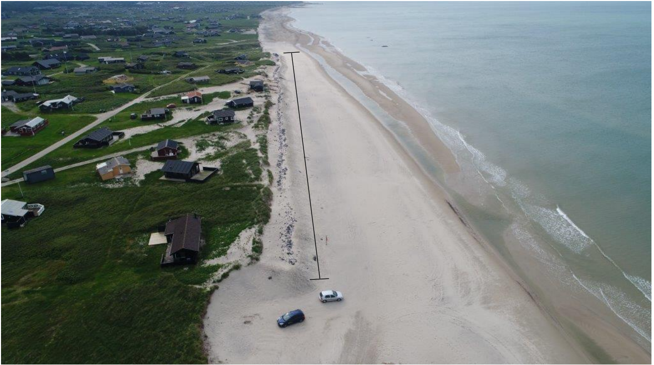
Figure 1.8 – A drone photo acquired in Noerlev beach, showing the newly installed sleeping defense. The black line is showing the extent of the revetment.
