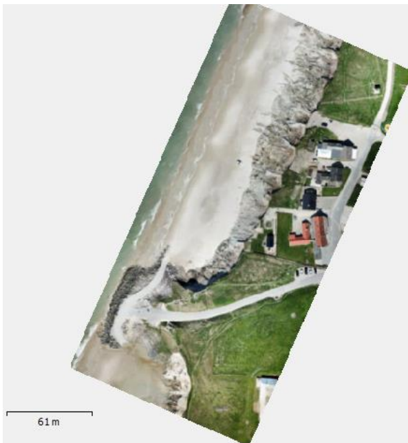
Figure 6.4 – Final Orthomosaic from the 14 th of May 2018. The resolution in the image is set to 0,04m.
