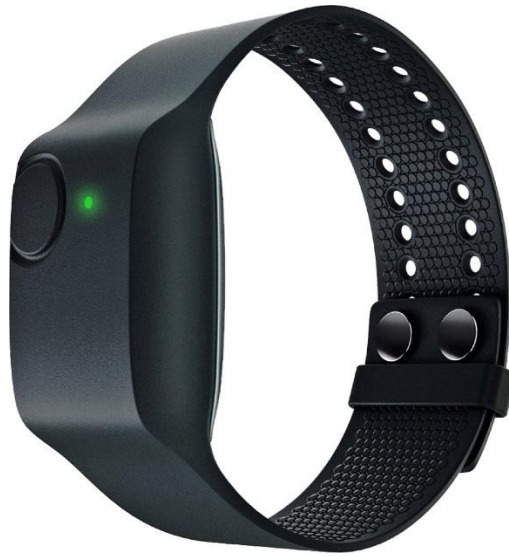
Figure 4.1 – Empatica Wrist Band used to measure GSR
