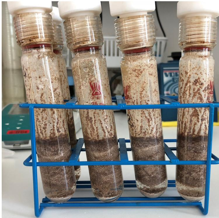
**Figure 6.6:** Example of emulsification phenomena in the test tubes
