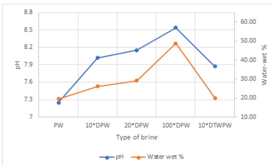
Figure 6.4: pH vs water-wetness for crude oil H
