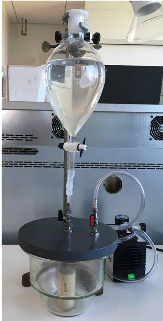
Figure 3.6: Volumetric funnel and desiccator for core saturation.
