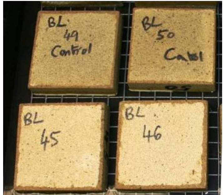
Figure 1 : Shows the appearance of the Blaxter sandstone blocks during the water absorption test.
