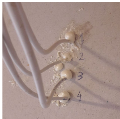
Figure 2.12: Sealed cavities for sensors inside the wall.
