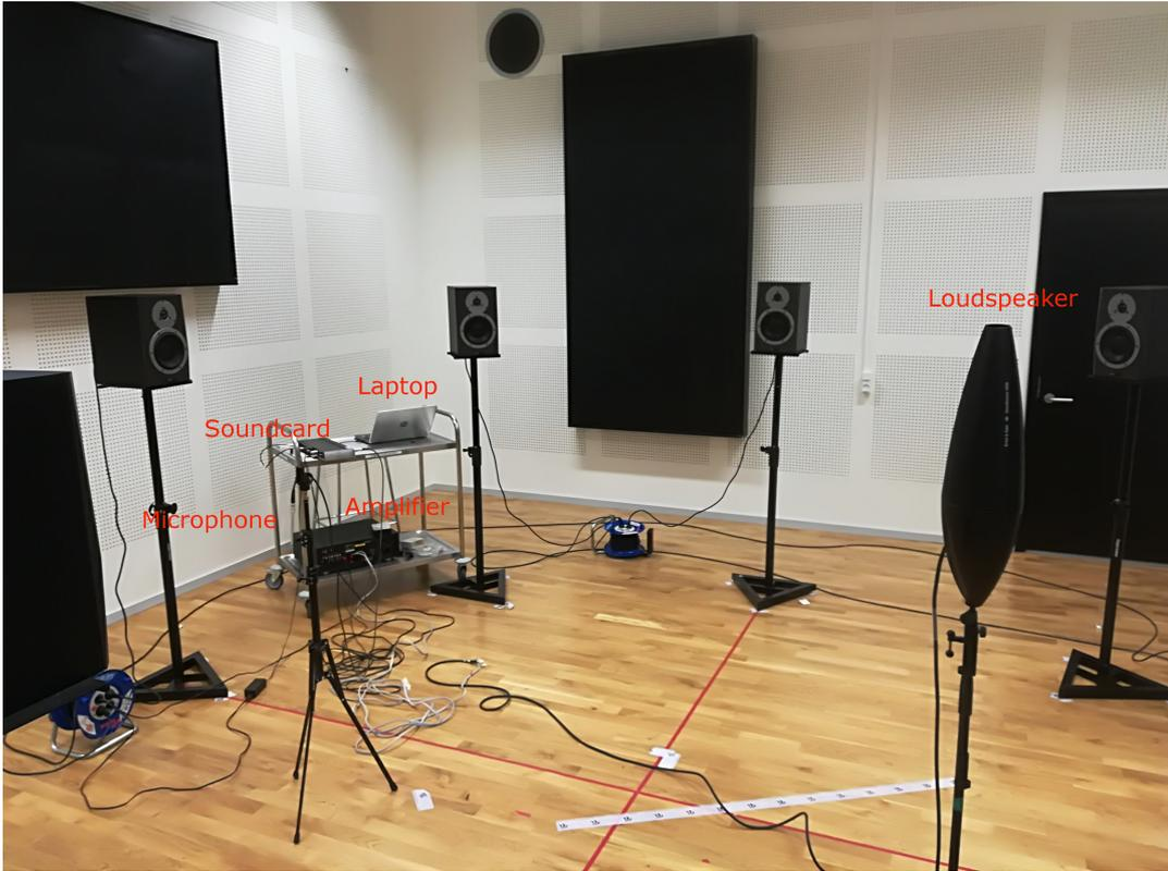
Figure C.1: RIR measurement set up sound lab
