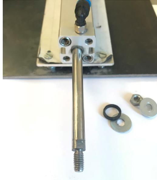
*Figure 4.6.* Close up of the actuator's mounting features.
