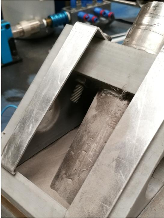
*Figure 4.14.* Powder in the filling shoe covering the brass plate.
