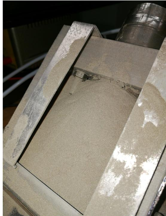
*Figure 4.15.* Filling shoe filled with powder.
