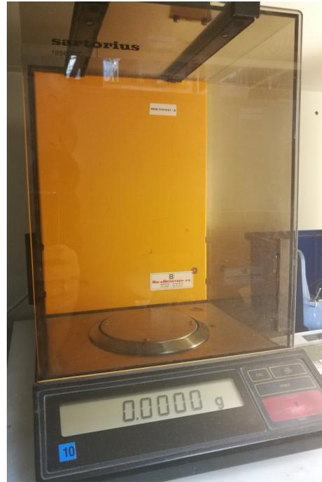
**Figure 4.21.** The scale used for measuring the average powder mass.
