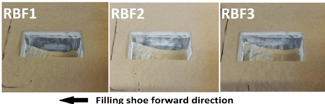
*Figure 5.12.* The filled dies of the three RBF experiments.
