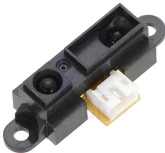
**Figure 4.11.** The distance measuring sensor.
