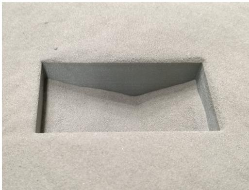
**Figure 3.14.** A close up picture of a not fully filled die.
