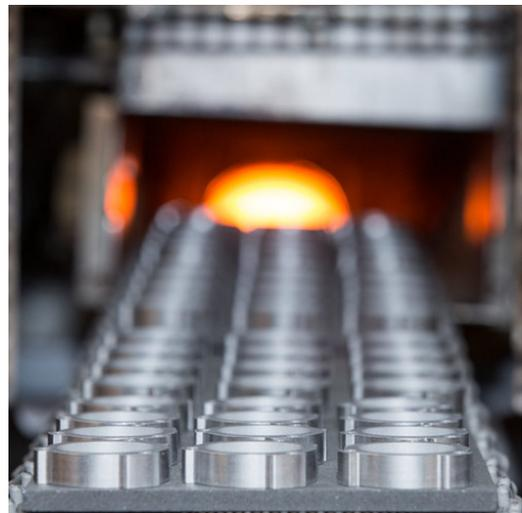
**Figure 2.7.** Parts entering the sintering furnace. Source: [1].
